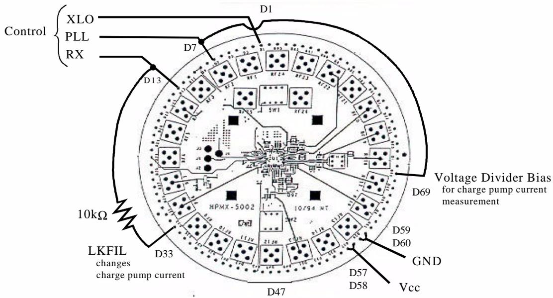
Note: User may prefer SW1 instead of external control lines D1, D7, and D13. In that case D1, D7, and D13 should be connected to Vcc. Also SW2 lines should be closed, i.e. shorted to ground.
