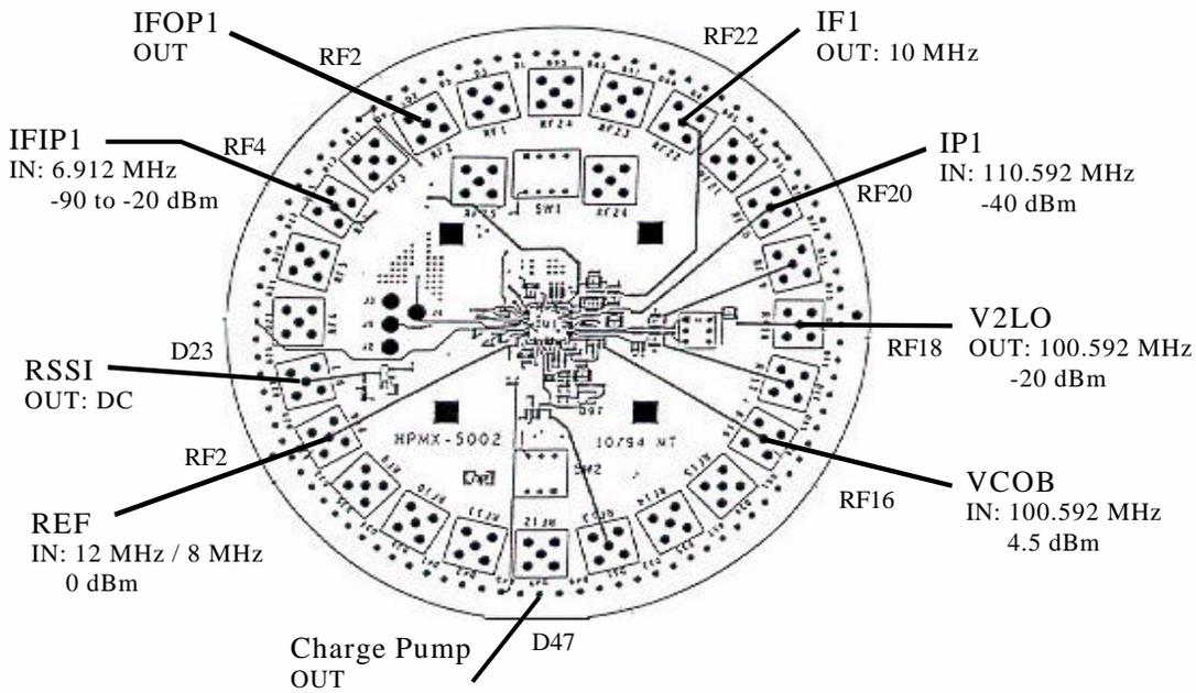
Figure 1: Signal Ports
