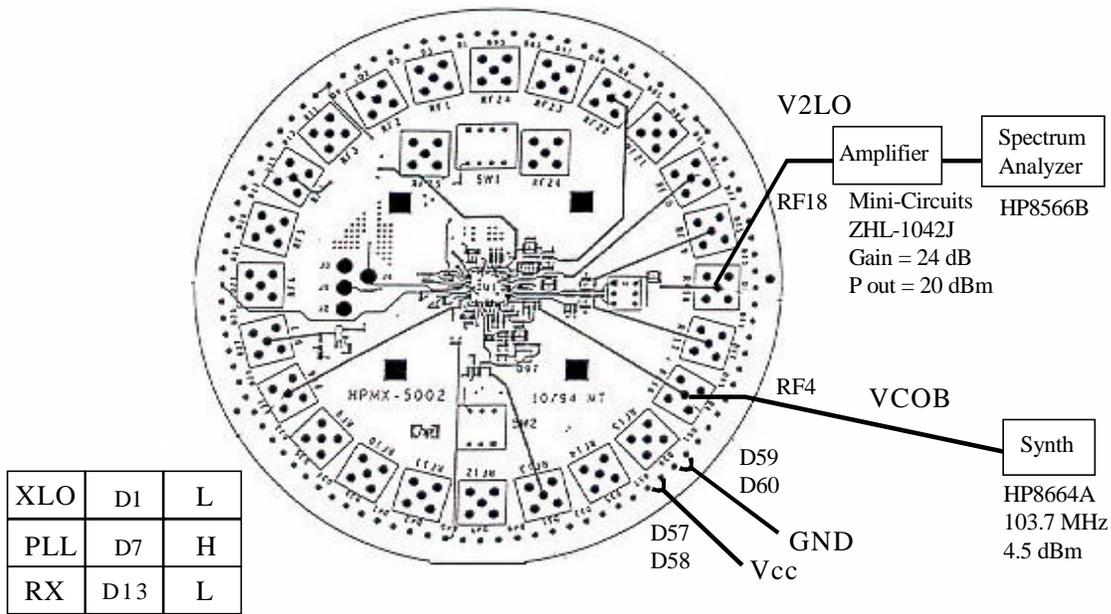
Figure 5: V2LO Noise Floor Measurement
