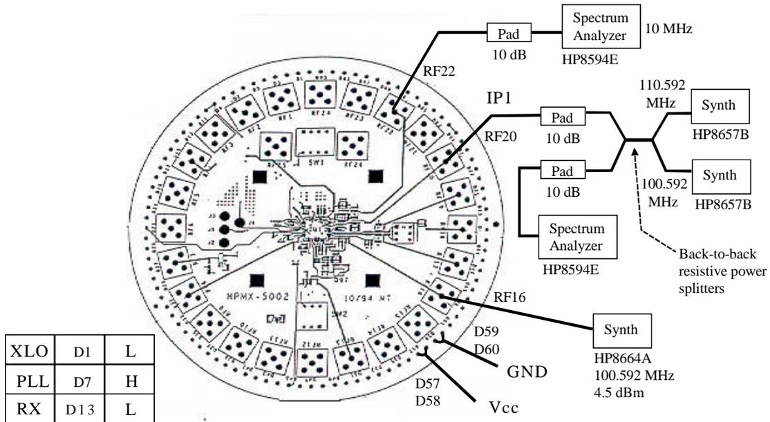
Figure3: Mixer IP3 Test
