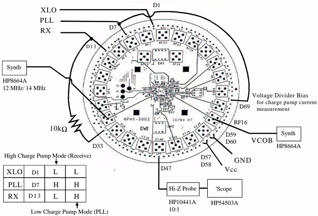
Figure 6: Charge Pump Test
