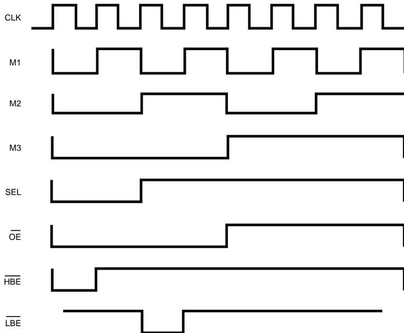
**Figure 3. Sequencer and Control Signals Timing Diagram.**
