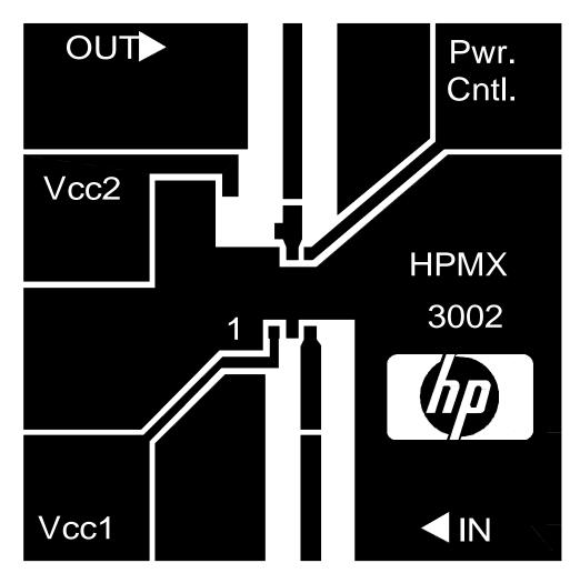
Fig. 2 Scale layout of demonstration circuit board.
