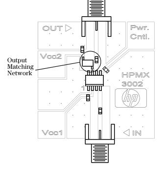
Figure 1. Assembled HPMX-3002 demonstration circuit board
