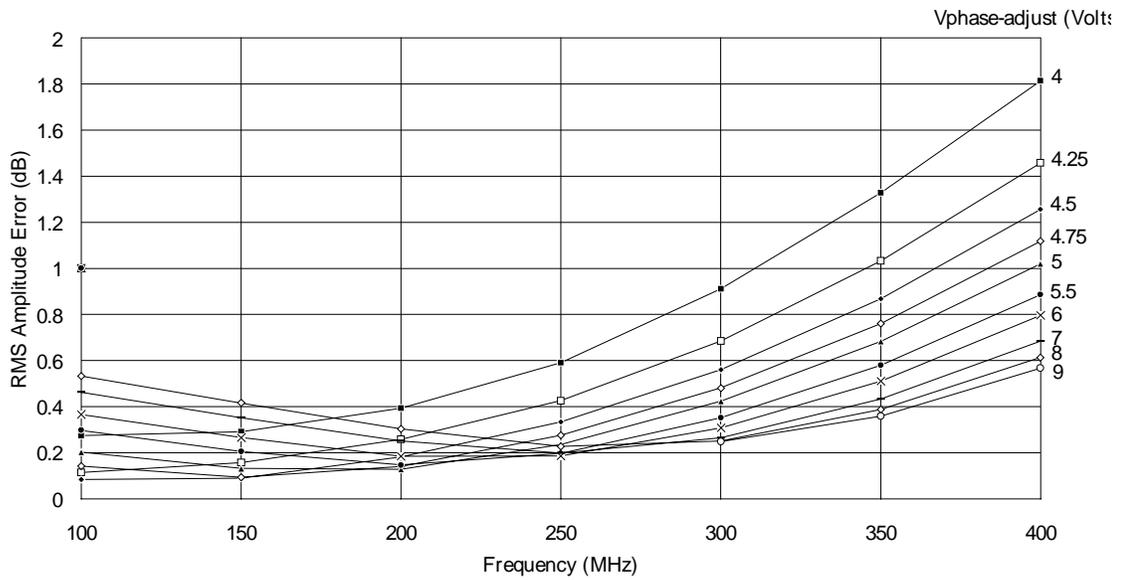
Figure 2. HPMX-2005 RMS Amplitude Error vs. Frequency and Vphase-adjust.
