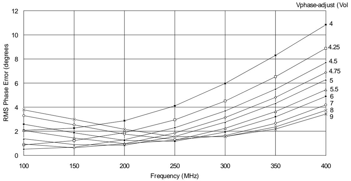
Figure 1. HPMX-2005 RMS Phase Error vs. Frequency and Vphase-adjust
