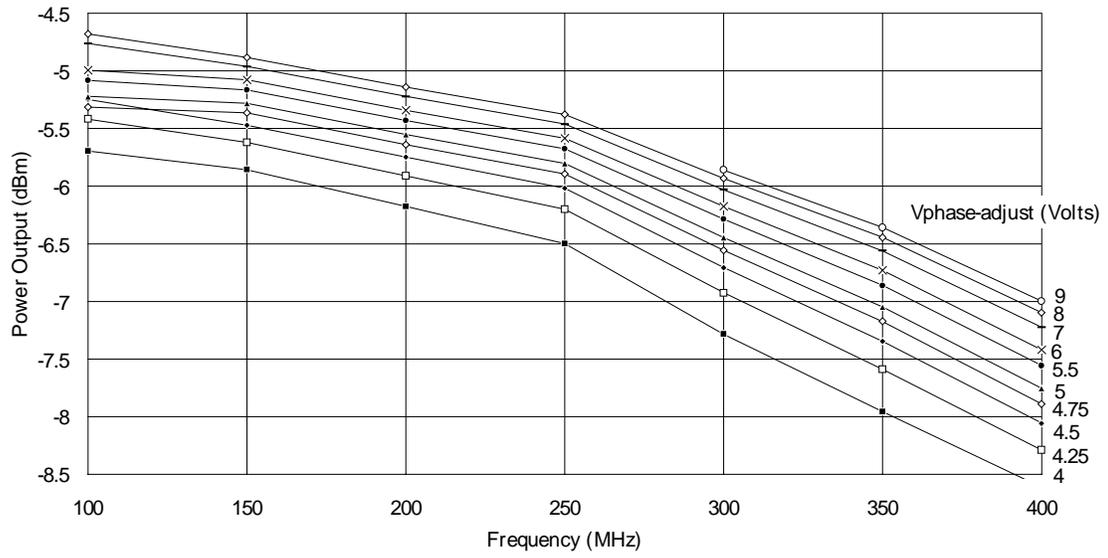
Figure 5. HPMX-2005 Power Output vs. Frequency and Vphase-adjust
