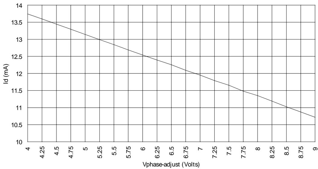
Figure 4. HPMX-2005 Device Current vs. Vphase-adjust
