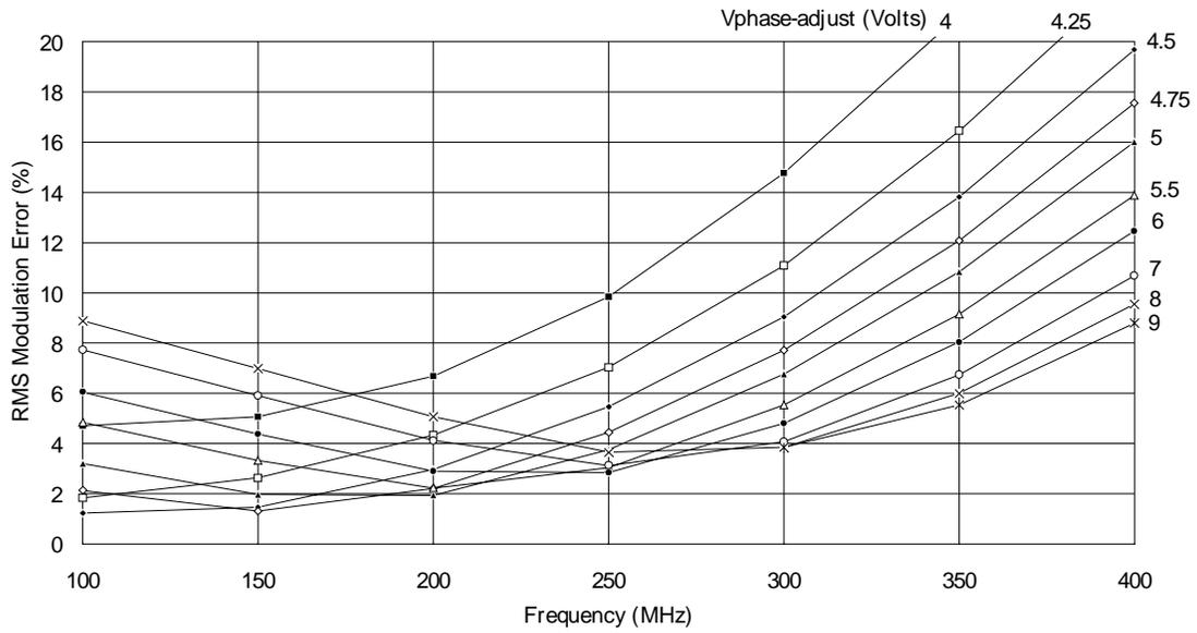
Figure 3. HPMX-2005 RMS Percent Modulation Error vs. Frequency and Vphase-adjust.
