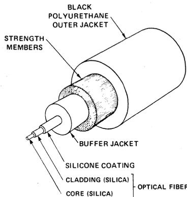
**Figure 6. Step Index Fiber Optic Cable Construction.**
