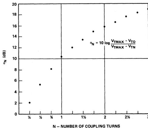
Figure 19. Flux Decoupling by Rotation of Connector Coupling.
