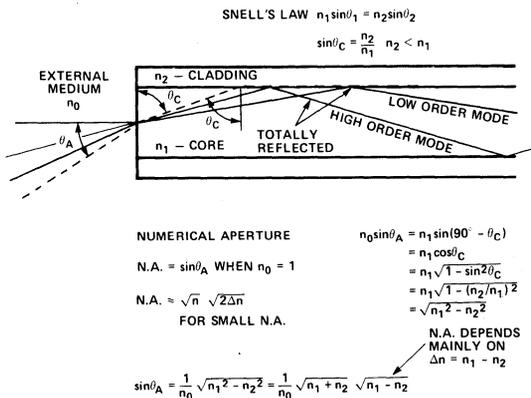
Figure 2. Total Internal Reflection.
