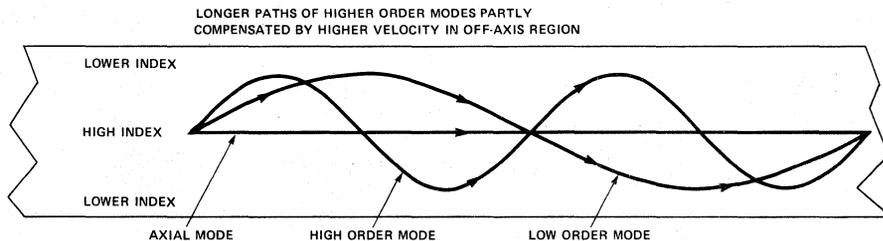
**Figure 5. Graded Index Fiber Modes.**
