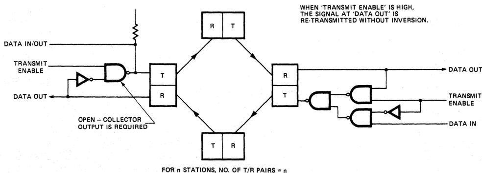
Figure 13. Looped-Station Multiplex Arrangement for Fiber Optic Links.
