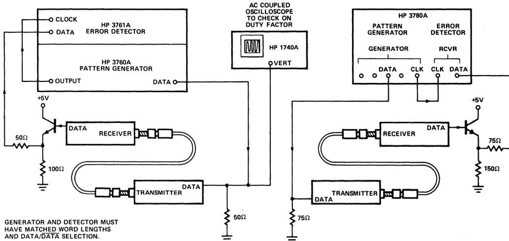
Figure 18. Bit Error Rate Measurement Arrangement.
