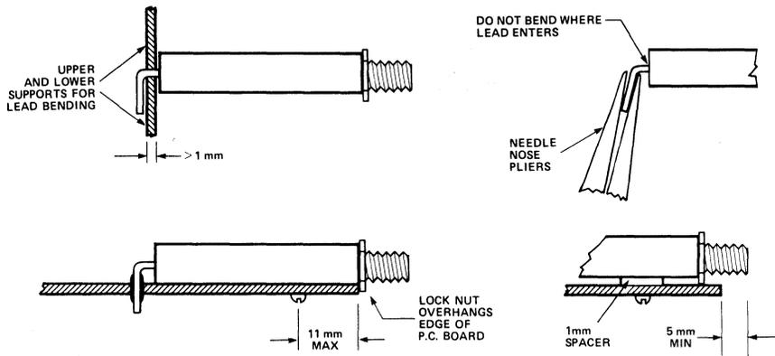
Figure 14. Lead Bending and P.C. Board Mounting.
