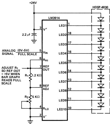
Figure 6. Low Power 0V-5V Bar Graph Meter
