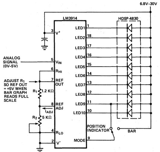
Figure 5. 0V-5V Bar Graph/Position Indicator Meter
