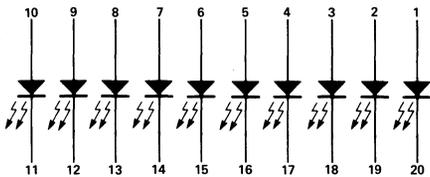
Figure 2. 10 Element Bar Graph Array Schematic
