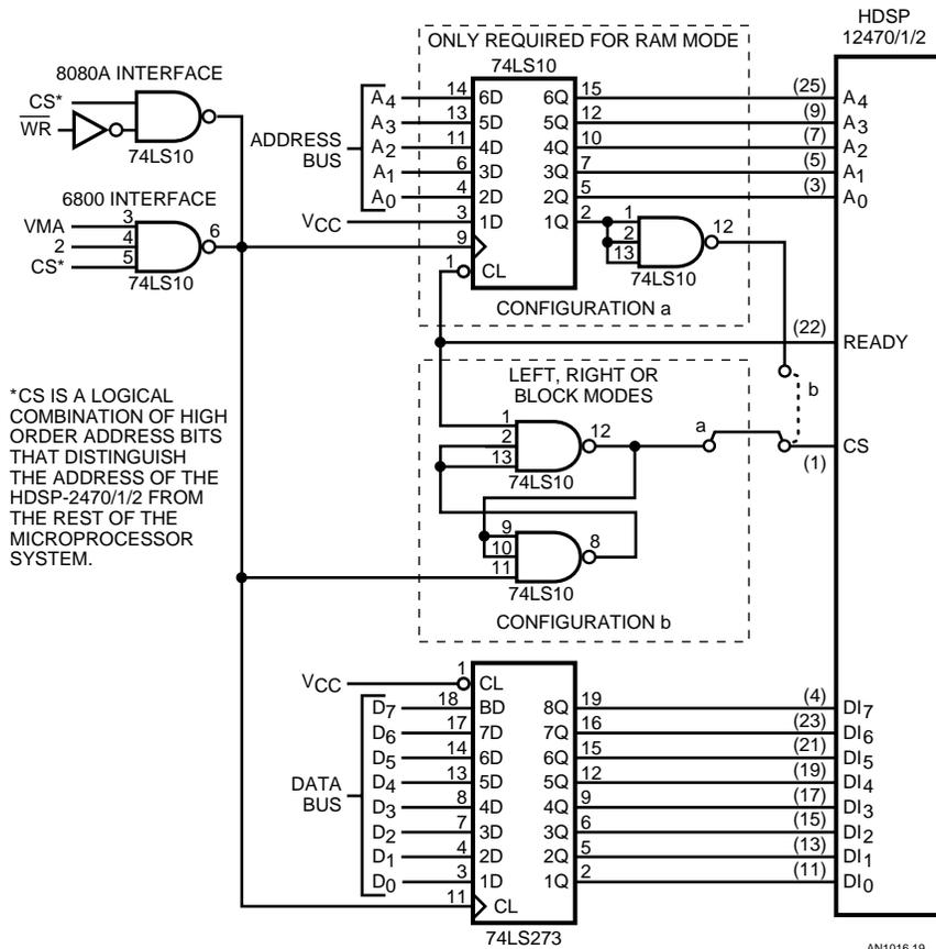
Figure 19. Latched Interface to the HDSP-2470/-2471/-2472 DISPLAY PROCESSOR CONTROLLER
