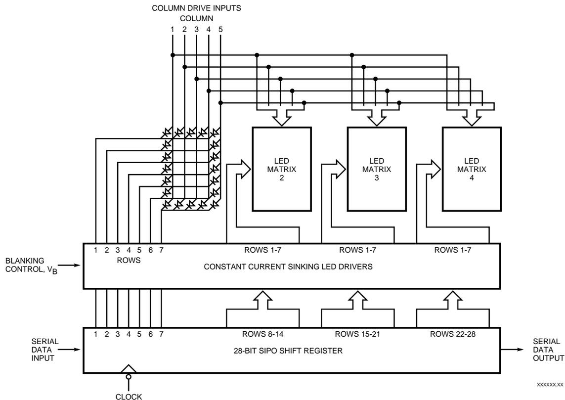
Figure 1. Block Diagram
