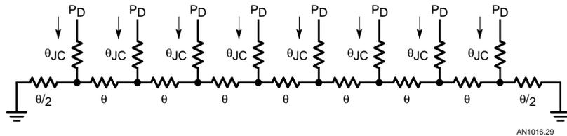
Figure 29. Thermal Resistance Model for Multiline HDSP-2000 Heat Sink
