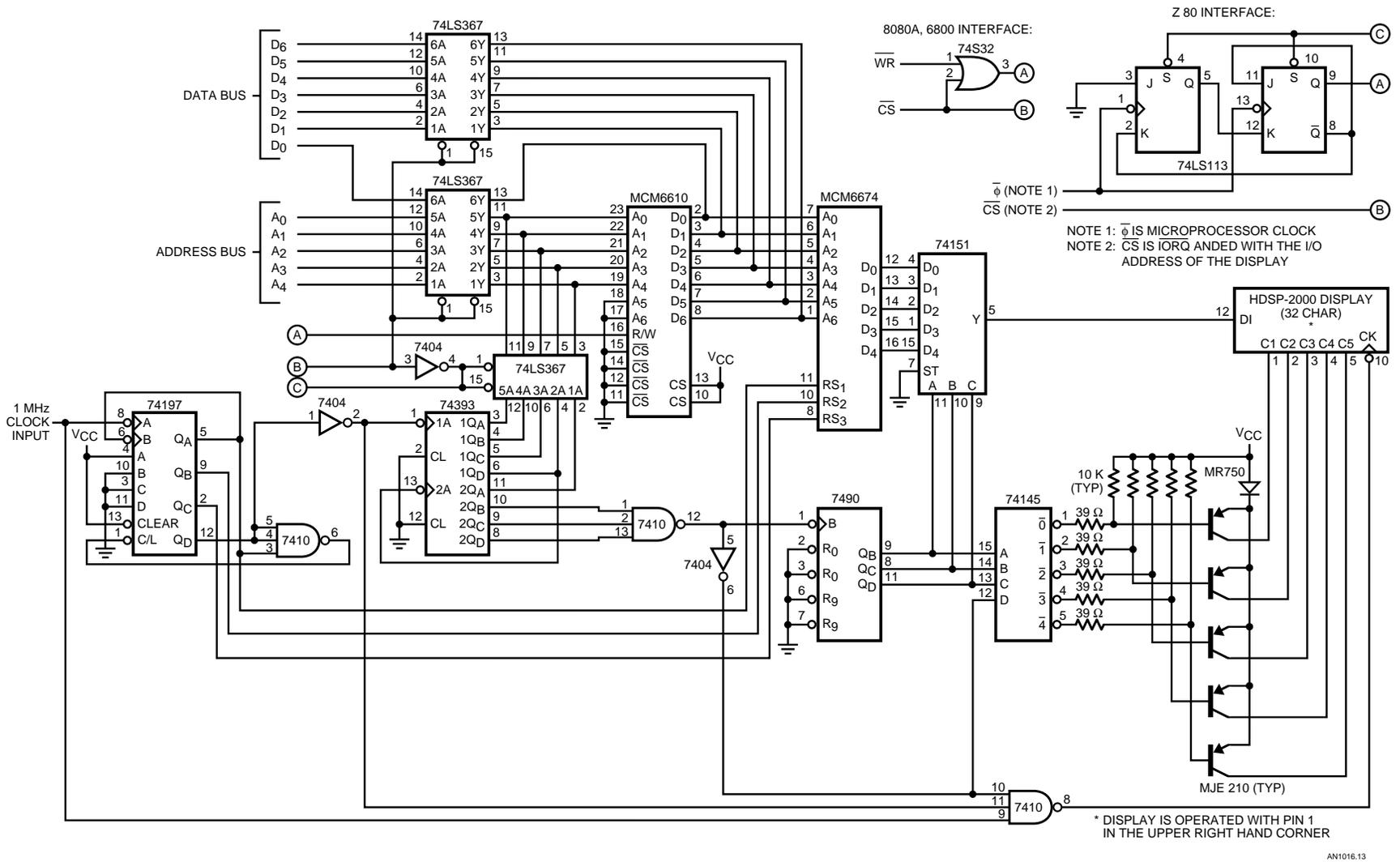
Figure 13. 8080A Microprocessor Interface to the 32 Character HDSP-2000 CODED DATA CONTROLLER
