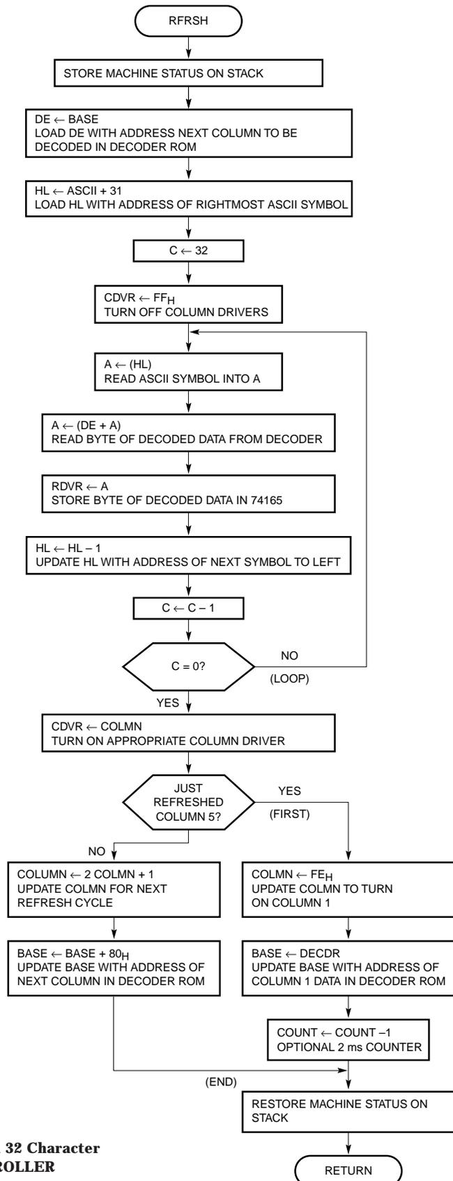
**Figure 8. 8080A Microprocessor Program that Decodes a 32 Character ASCII String Prior to Loading into the REFRESH CONTROLLER**
