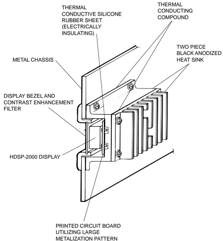
Figure 27. Two-Part Heat Sink for the HDSP-2000
