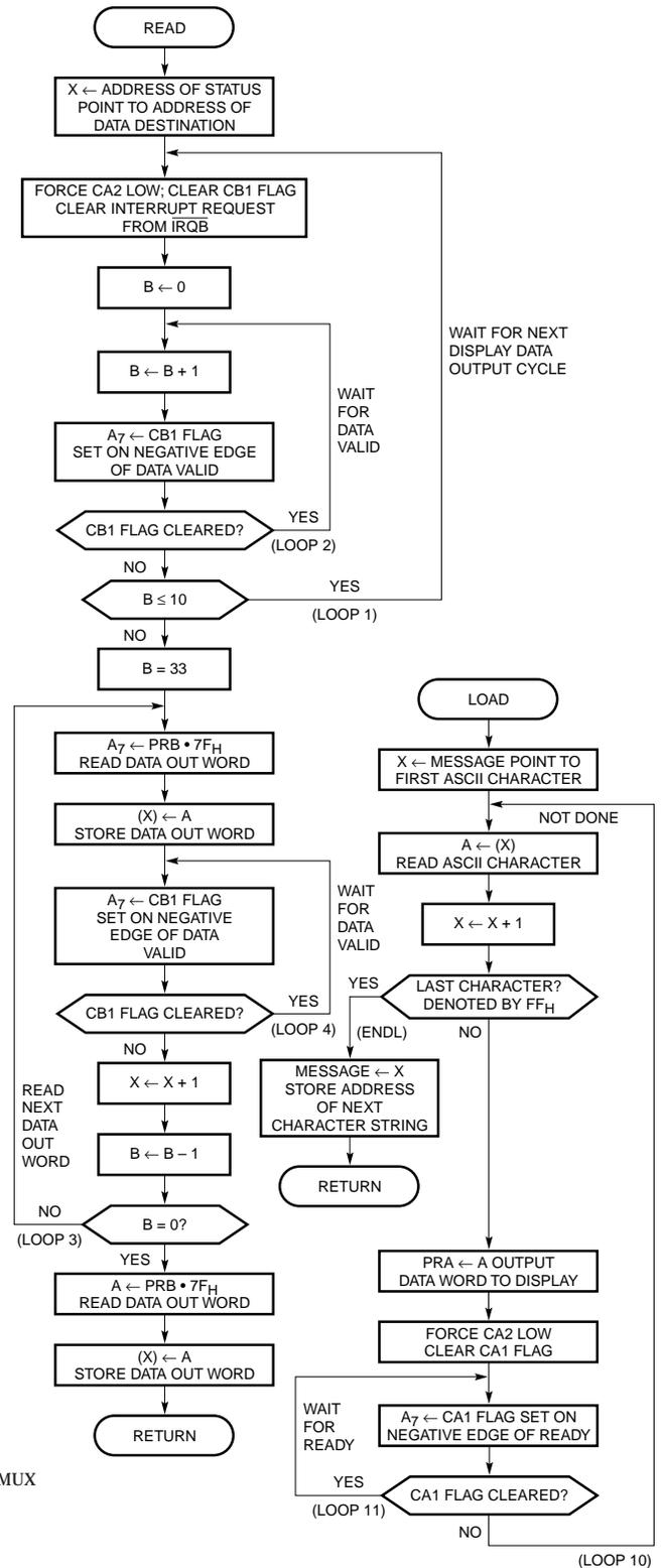
Figure 21. 6800 Microprocessor Program that Interfaces to the Circuit shown in Figure 14.
