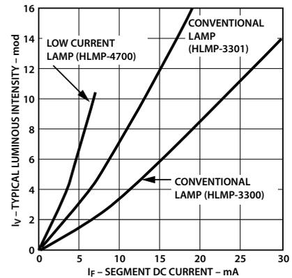
Figure 1. Typical Luminous Intensity vs. Forward Current
