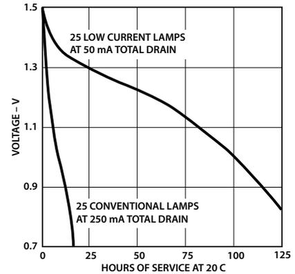
Figure 8. Typical "C" Cell Discharge Characteristics
