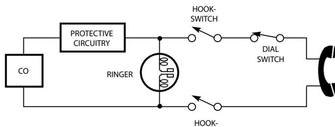
Figure 7. Simplified Telephone Diagram
