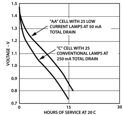
Figure 9. Typical "AA" and "C" Cell Discharge Characteristics
