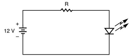
Figure 5. Lamp Circuit Using 12 Volt DC Supply
