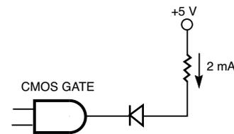
Figure 4. Circuit to Drive a Low Current Lamp
