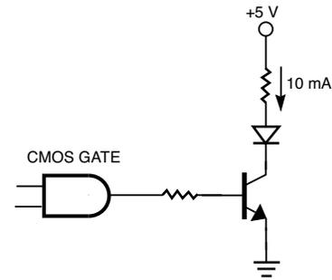
Figure 3. Circuit to Drive a Conventional Lamp
