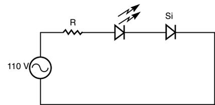
Figure 6. Lamp Circuit Using 110 Volt AC Supply
