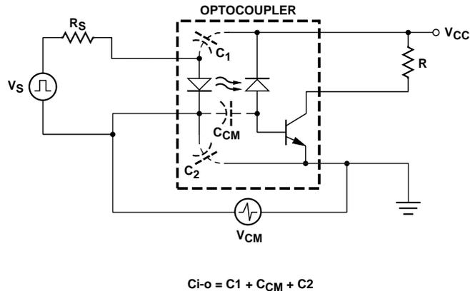
**Figure 5. Input-to-Output Capacitance.**
