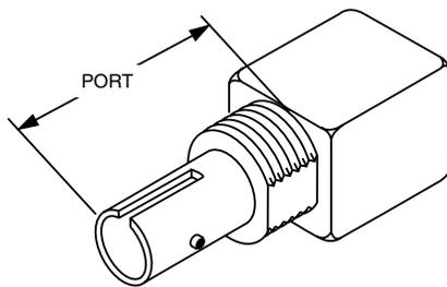
Figure 1. Fiber Optic Receiver
