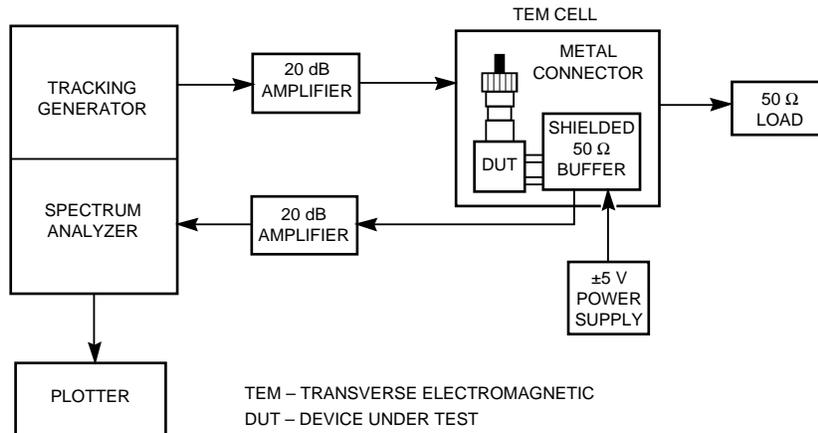
**Figure 3. Block Diagram of Test Setup for Electromagnetic Susceptibility.**
