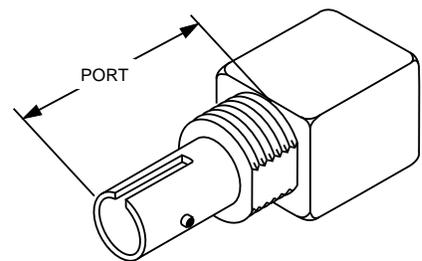
**Figure 1. Fiber Optic Receiver.**
