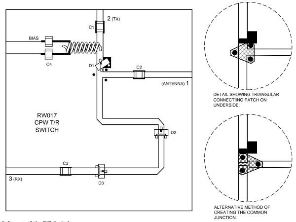
Figure 8. Layout of the T/R Switch.
