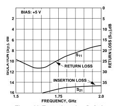
Figure 11. Transmitter Arm Isolation. minimize the number of different diode part numbers kept in stock.
