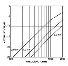
Figure 2. Attenuation vs. Frequency, Inductor Shunting a 50  $\Omega$  line.
