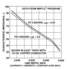
Figure 5. Impedance vs. Linewidth, CoPlanar Waveguide.
