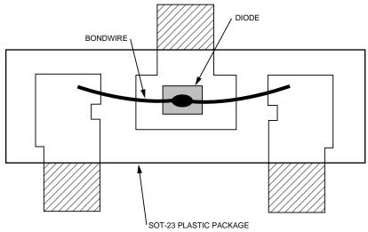
Figure 3. HSMP-4890 Low Inductance Diode.
