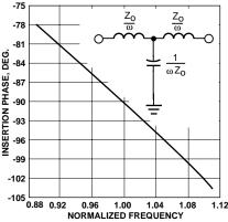
Figure 6. 90° Phase Delay Circuit.
