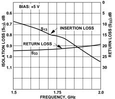
Figure 12. Receiver Arm Insertion Loss. concepts based upon CoPlanar Waveguide and a new, low inductance PIN diode. The design approach contained in this paper is easily scaled to other frequency ranges.
