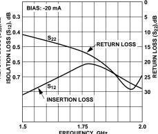
Figure 13. Transmitter Arm Insertion Loss.
