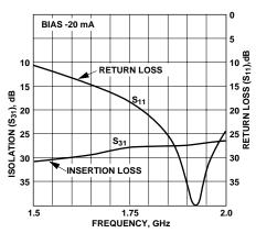
Figure 10. Receiver Arm Isolation.
