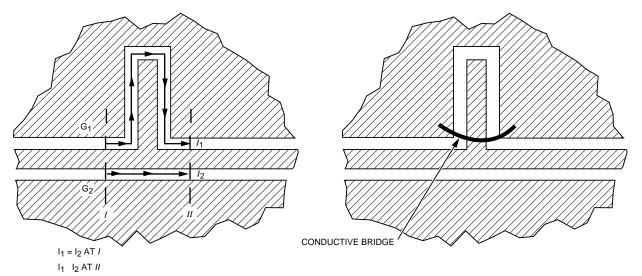
Figure 17. Control of Ground Currents in CPW.
