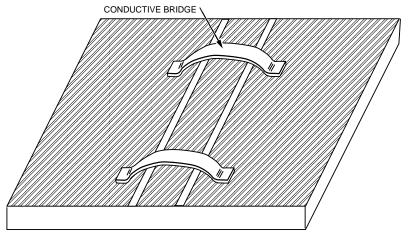
Figure 16. CPW with Conductive Bridge.
