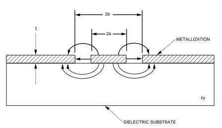
Figure 14. Cross-Section of CoPlanar Waveguide.
