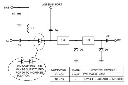
Figure 7. Schematic of the prototype Switch.
