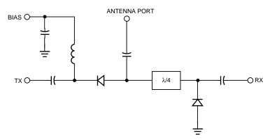
Figure 1. Low Current T/R Switch.
