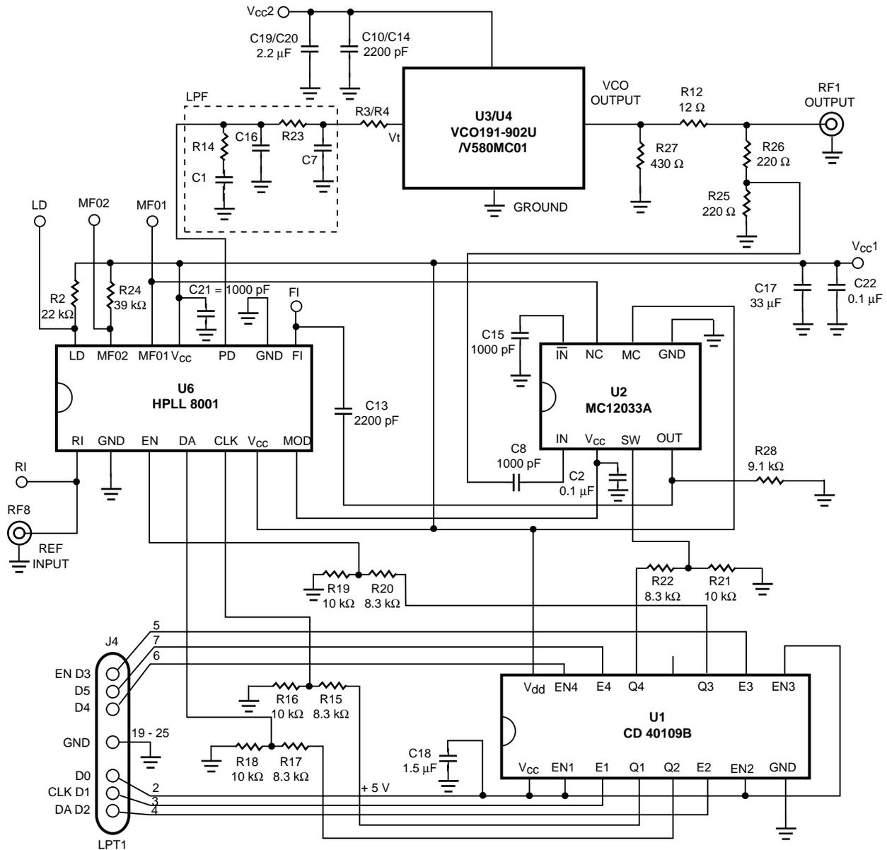
Figure 2. PLL Frequency Synthesizer Schematic
