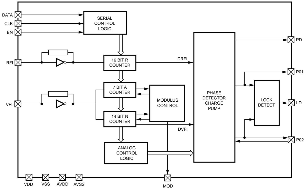
**Figure 1. HPLL-8001 Internal Block diagram**
