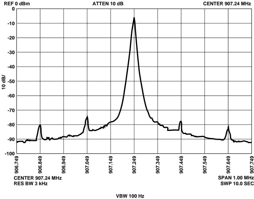
Figure 4. Typical GSM Spectrum Plot
