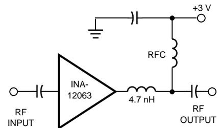
**Figure 1. RF Schematic of 2.4 GHz Amplifier**
