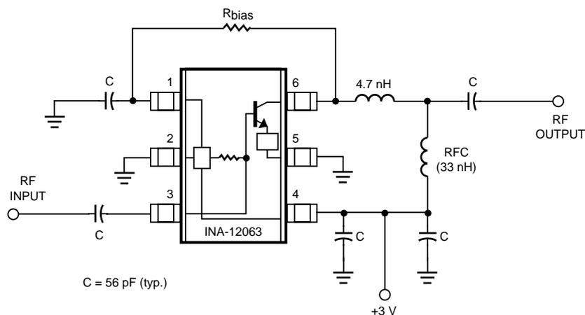
Figure 4. Complete Schematic of 2.4 GHz Amplifier
