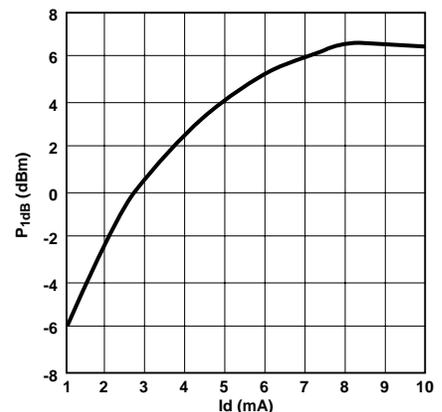
Figure 7. Output Power ( $P_{1dB}$ ) vs. Device Current
