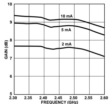
**Figure 2. Gain of 2.4 GHz Circuit Using INA-12063**
