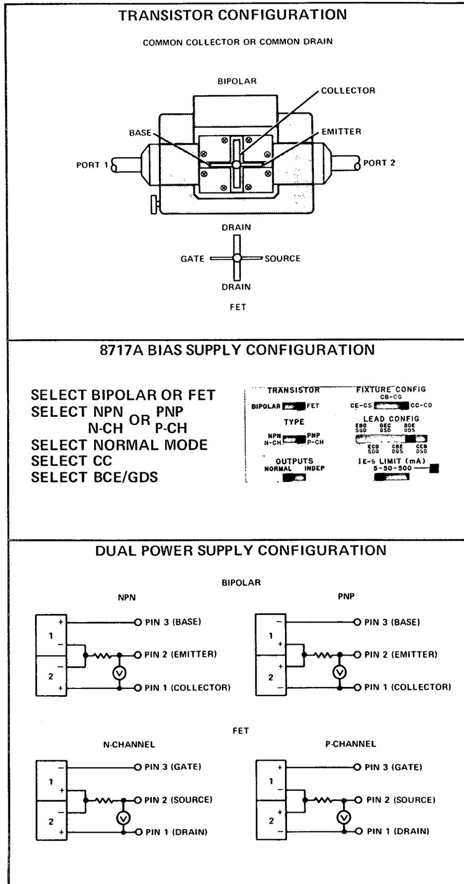
Figure 13. Bias Supply Configuration for Common Collector
