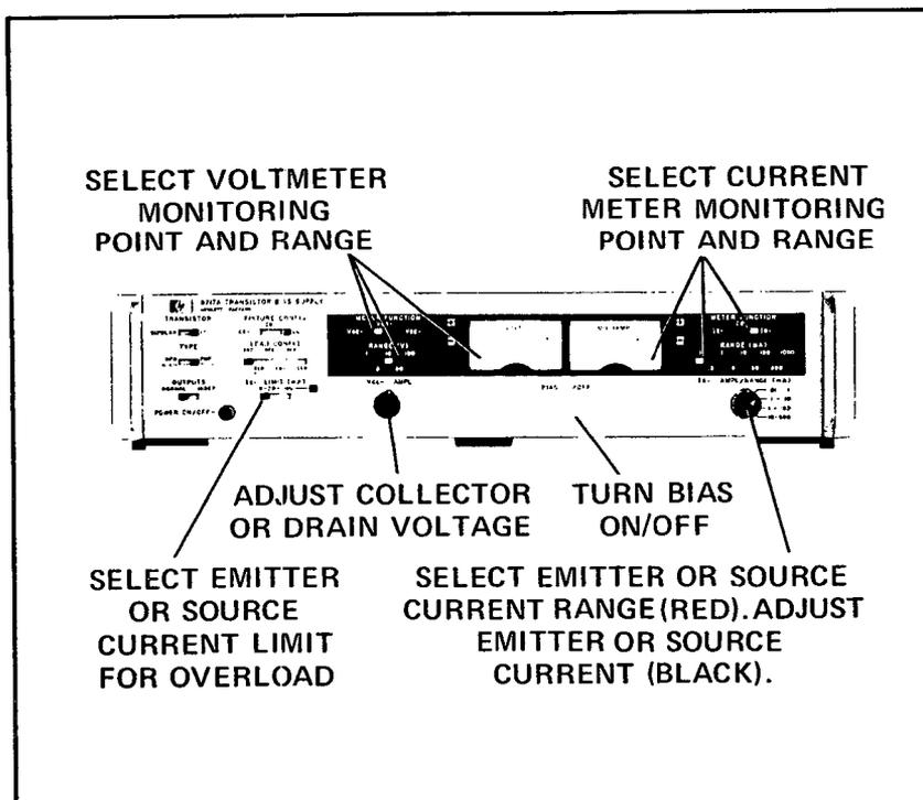
Figure 10. Operating Controls of the 8717A Power Supply
