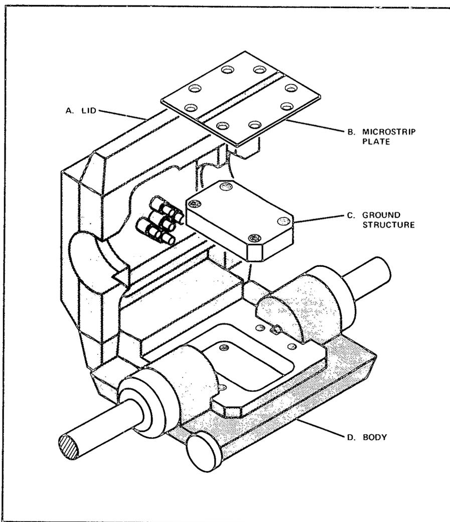
Figure 15. An Exploded View of the 11608A Test Fixture with Option 001
