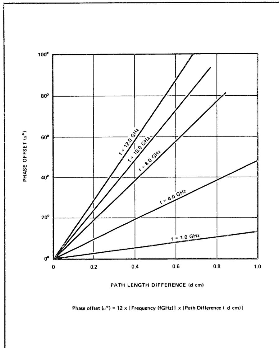
Figure 18. Linear Phase Offset as a Function of Path Length and Frequency
