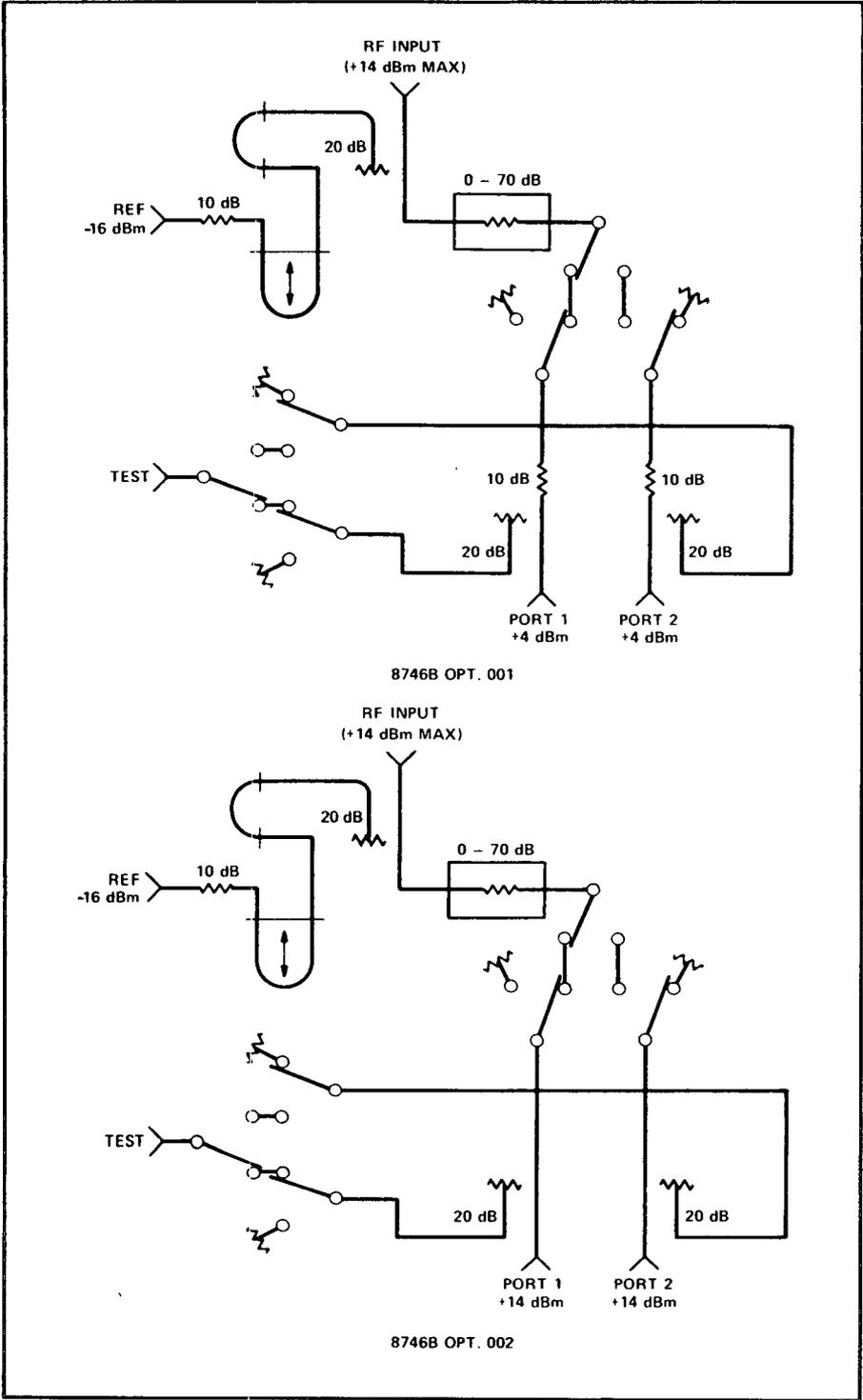
Figure 5. Simplified Block Diagram of Options 001 and 002
