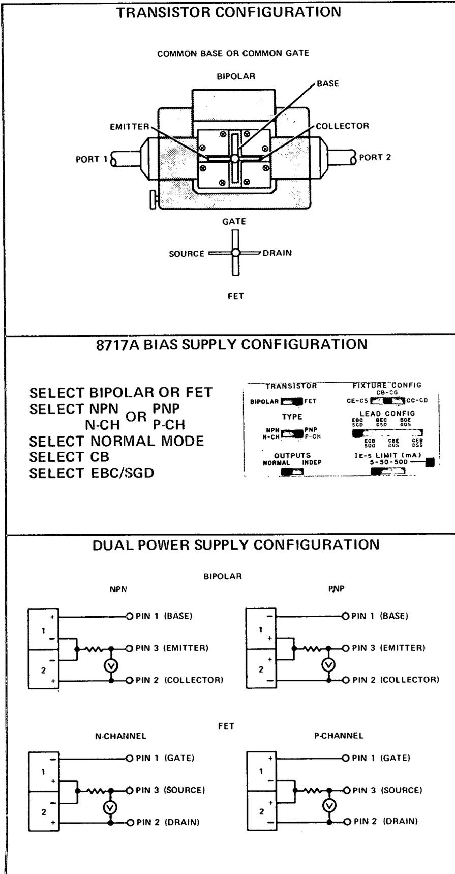
Figure 12. Bias Supply Configuration for Common Base
