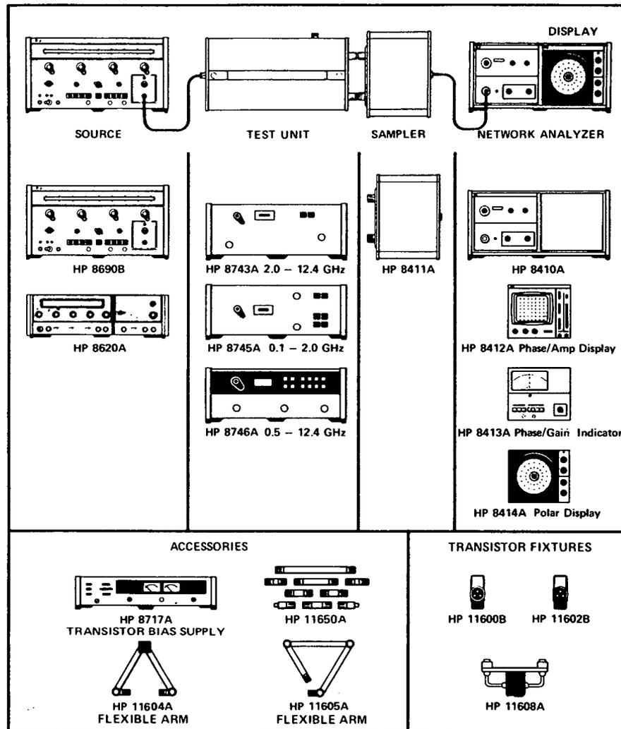
Figure 1. Network Analyzer System Components
