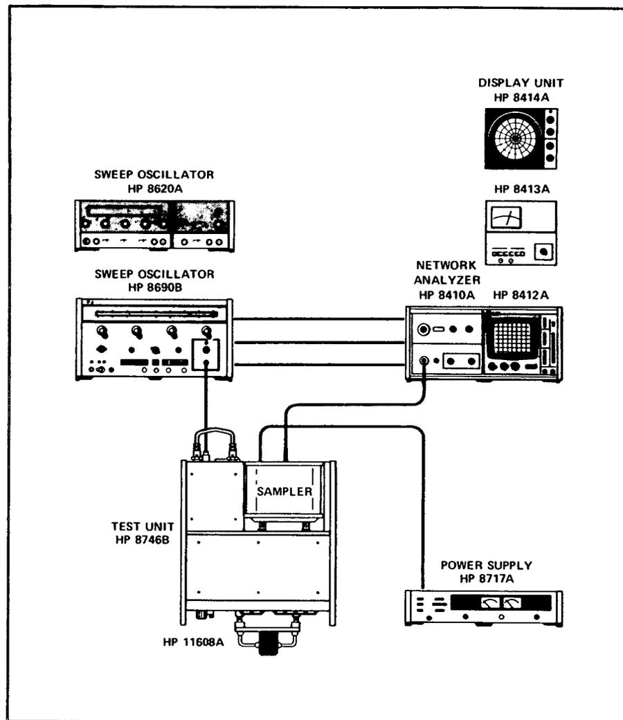
Figure 3. System Configuration for Stripline Measurements
