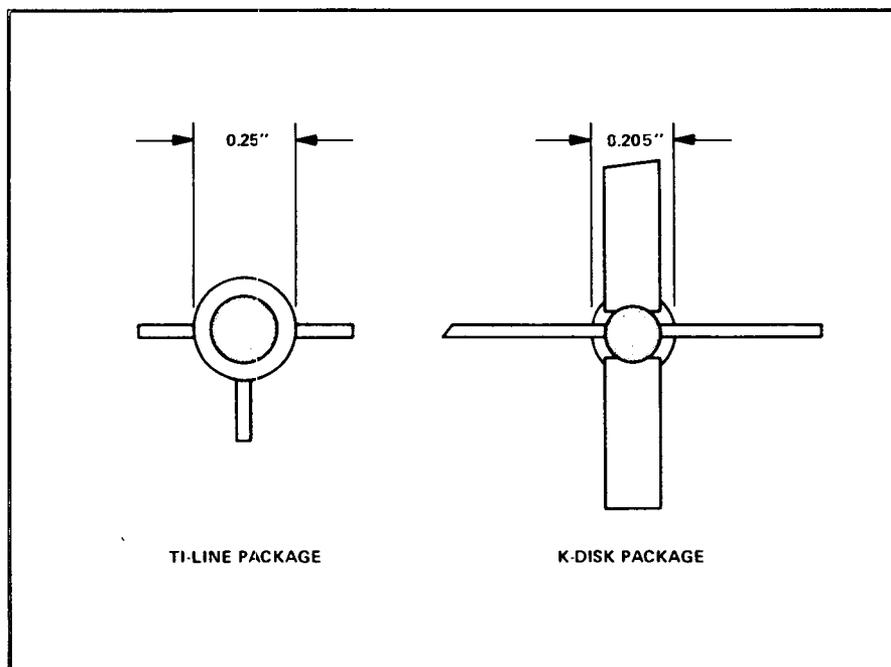
*Figure 6. TI-Line and K-Disc Package Styles*
