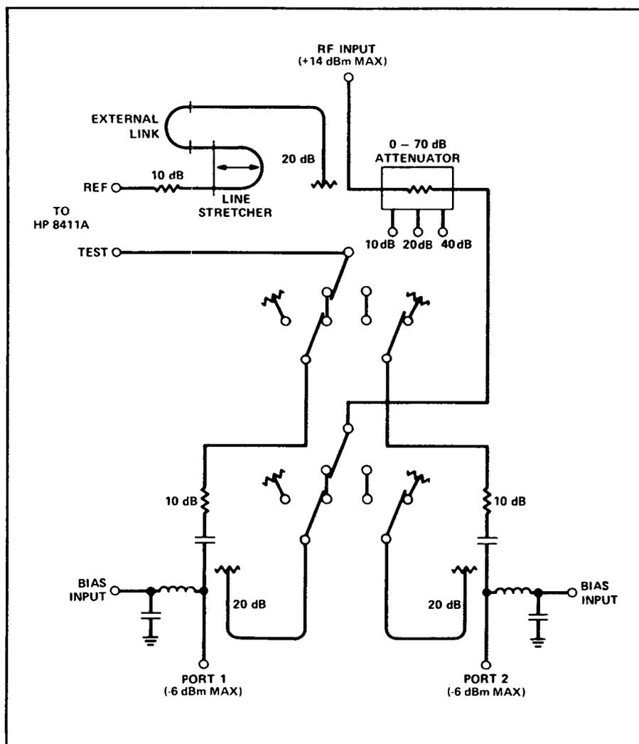
Figure 4. Simplified Block Diagram of the 8746B
