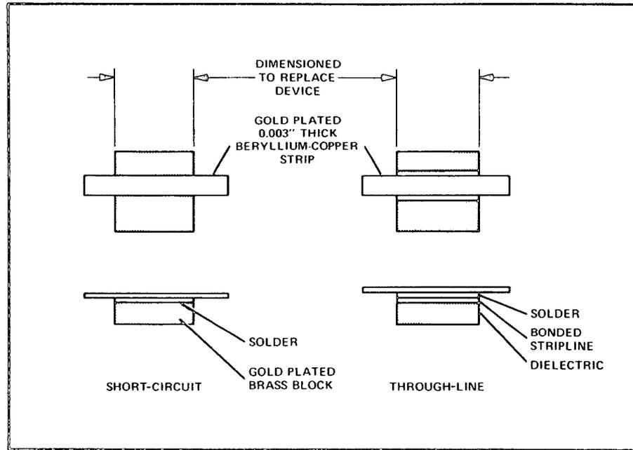
Figure 17. Typical Short Circuit and Through Line Calibration Units
