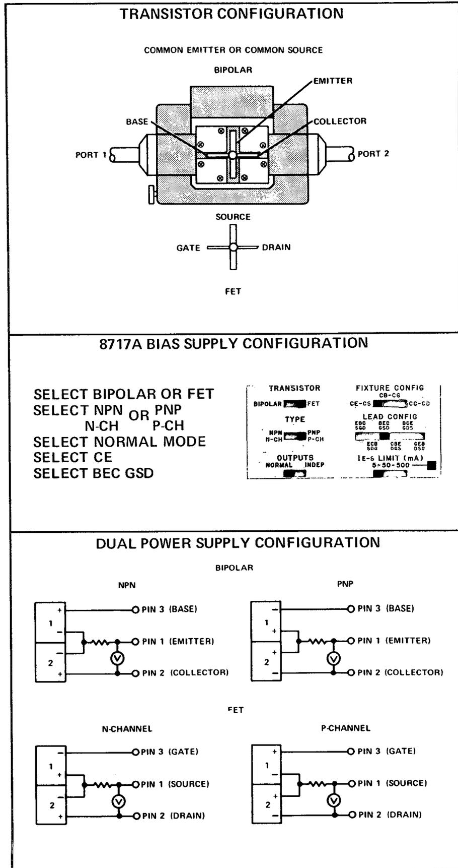
Figure 11. Bias Supply Configuration for Common Emitter
