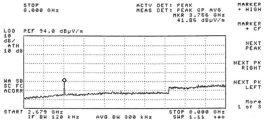
Figure 11. Worst Case Reference Board EMI with four HFCT-5912E's was 41.9d B $\mu$ V/m @ 3.756 GHz
