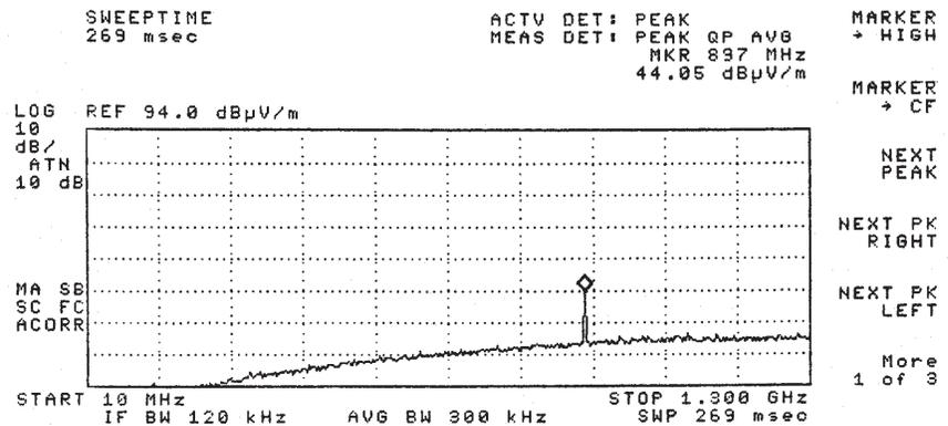
Figure 12. Worst Case Reference Board EMI with four HFBR-5912E's was 44.1d B $\mu$ V/m @ 897 MHz
