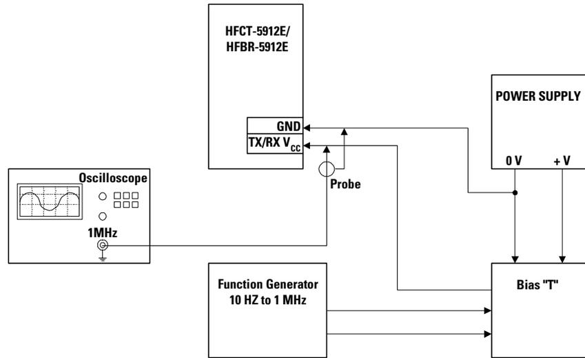
Figure 9. Power Supply Noise Immunity Test Setup
