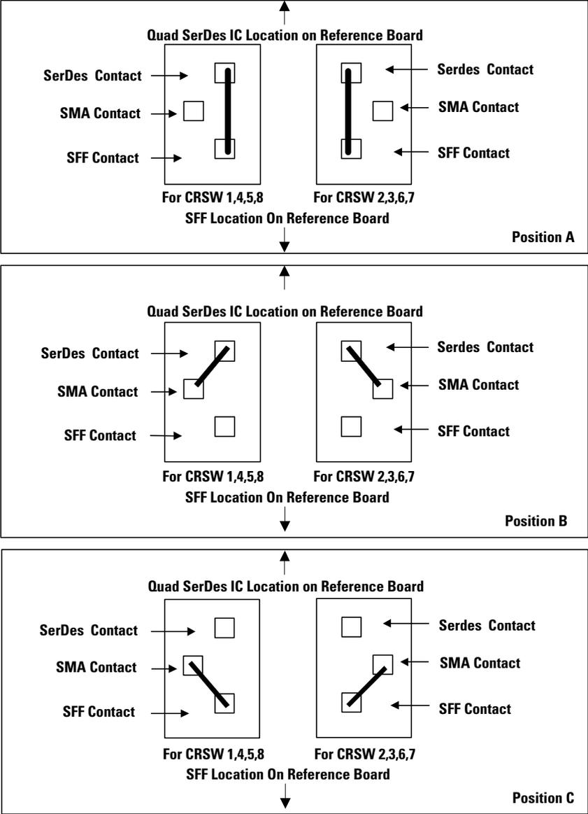
Figure 3. User Available Test Options For Channels U2 and U5.
