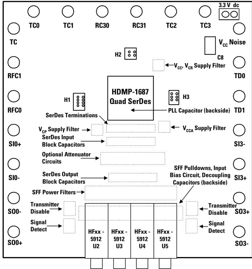
Figure 1. Main Components of the Reference Board
