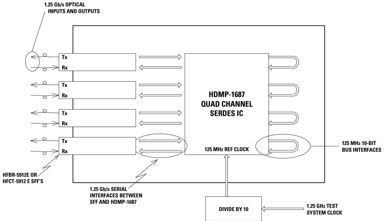
Figure 2. Block Diagram of the Reference Board
