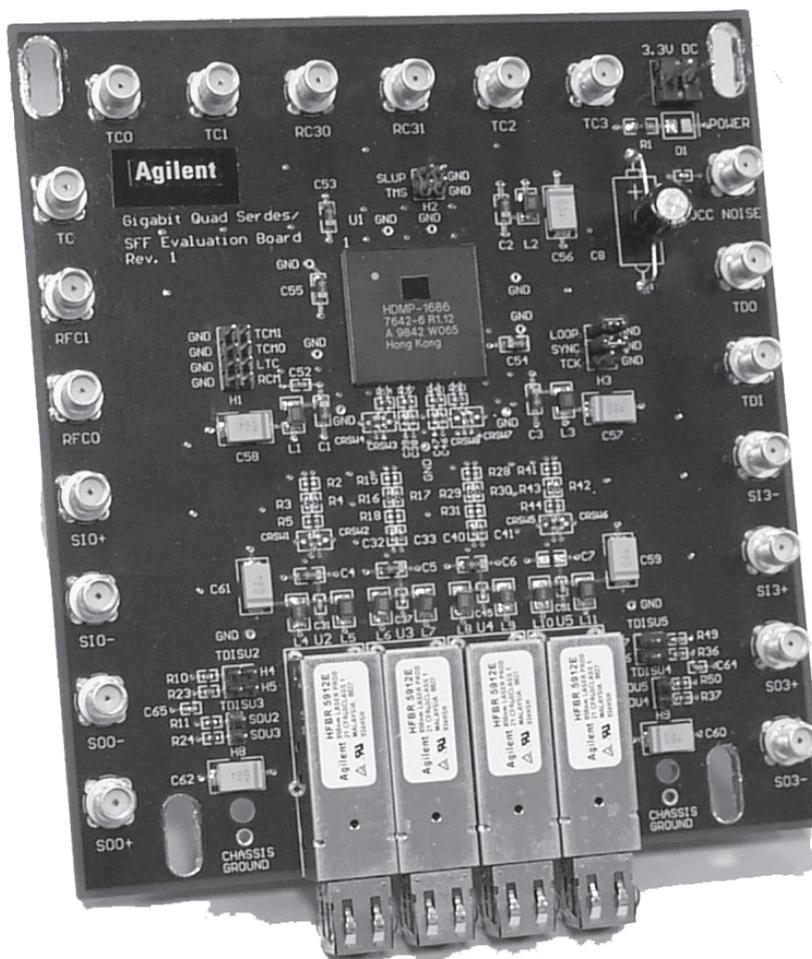
specification for IEEE 802.3z Gigabit Ethernet. For more information on this component reference should be made to the Agilent technical data sheet.
