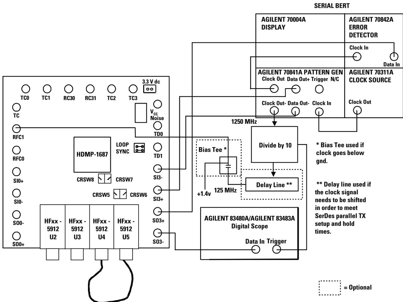
Figure 4. Test Setup with Reference Board
