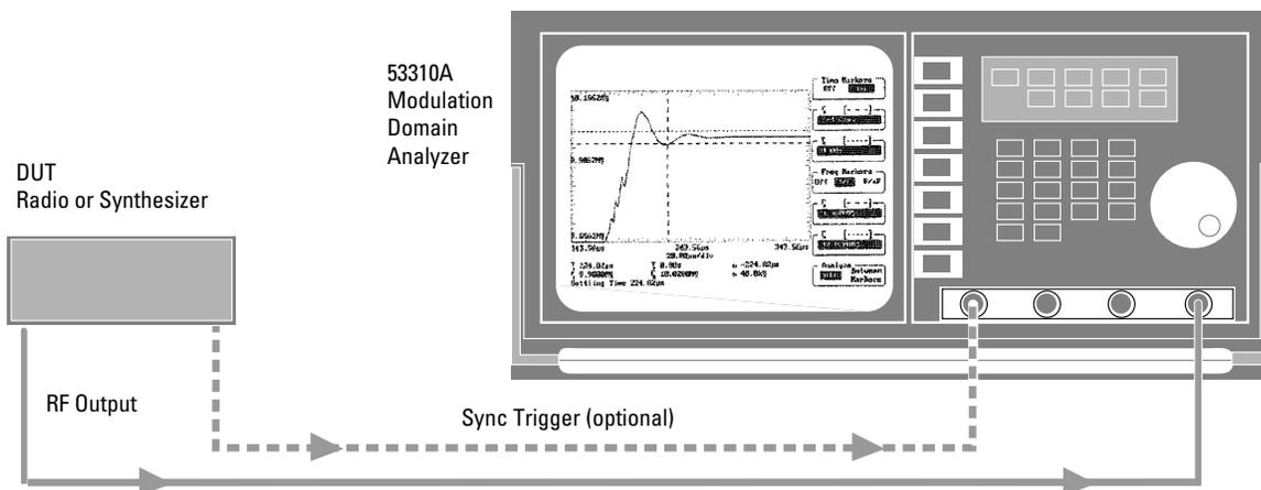
Figure 5. Direct connection makes measurement setup easy.
