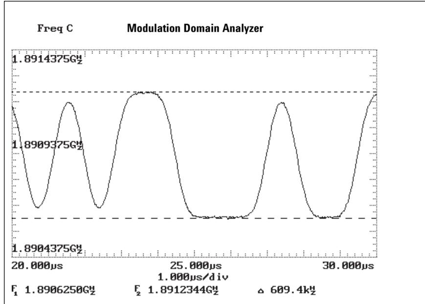
Figure 8. The high resolution RF input directly profiles the FSK modulation on a DECT signal.
