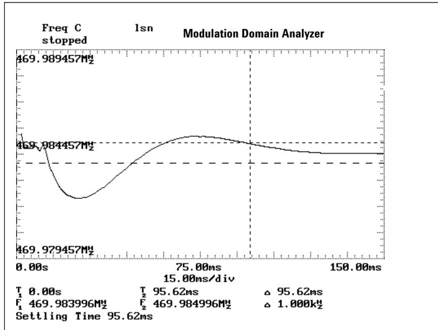
Figure 7. Frequency turn-on behavior of a mobile radio viewed directly on a modulation domain analyzer.
