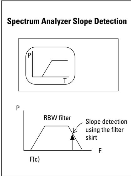
**Figure 2. The slope detection method with a spectrum analyzer offers limited accuracy because of filter nonlinearity.**
