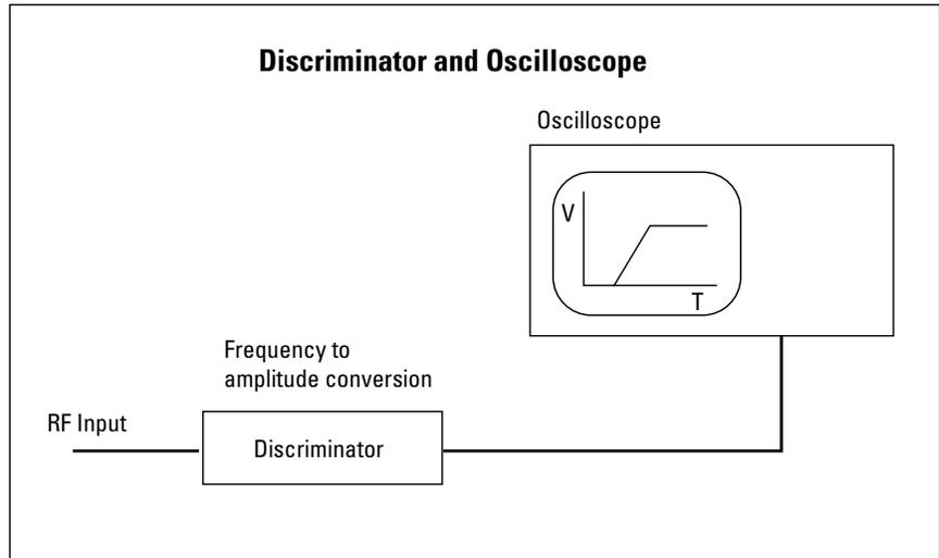
**Figure 1. Using a discriminator for measuring synthesizer settling time does not provide calibrated, repeatable results.**
