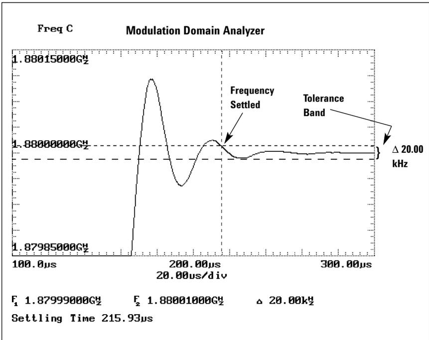
**Figure 3. A modulation domain analyzer provides highly accurate automatic measurements of synthesizer settling time.**
