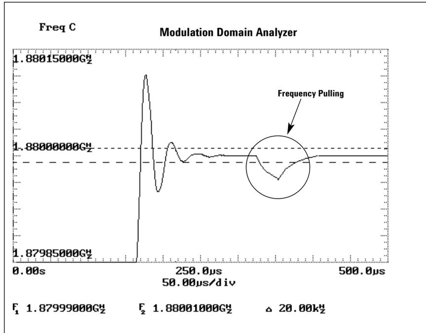
Figure 4. Frequency pulling effects can easily be seen using a modulation domain analyzer.
