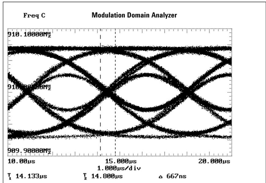
Figure 9. Frequency-versus-time eye diagrams make it easy to view jitter effects on the RF carrier.
