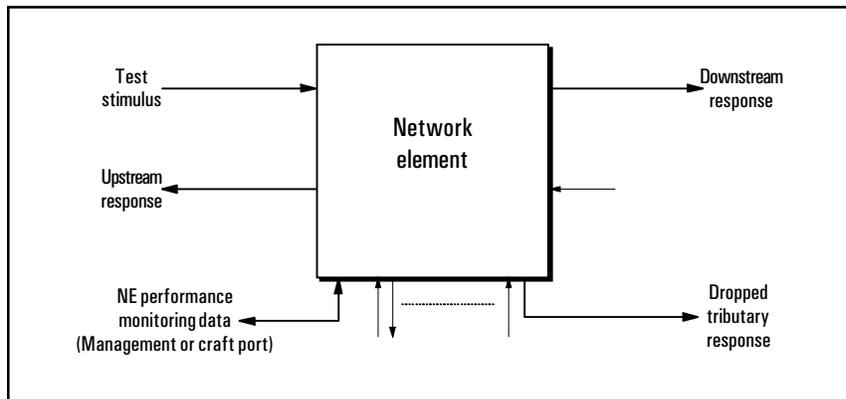
Figure 1. Connecting to network element under test
