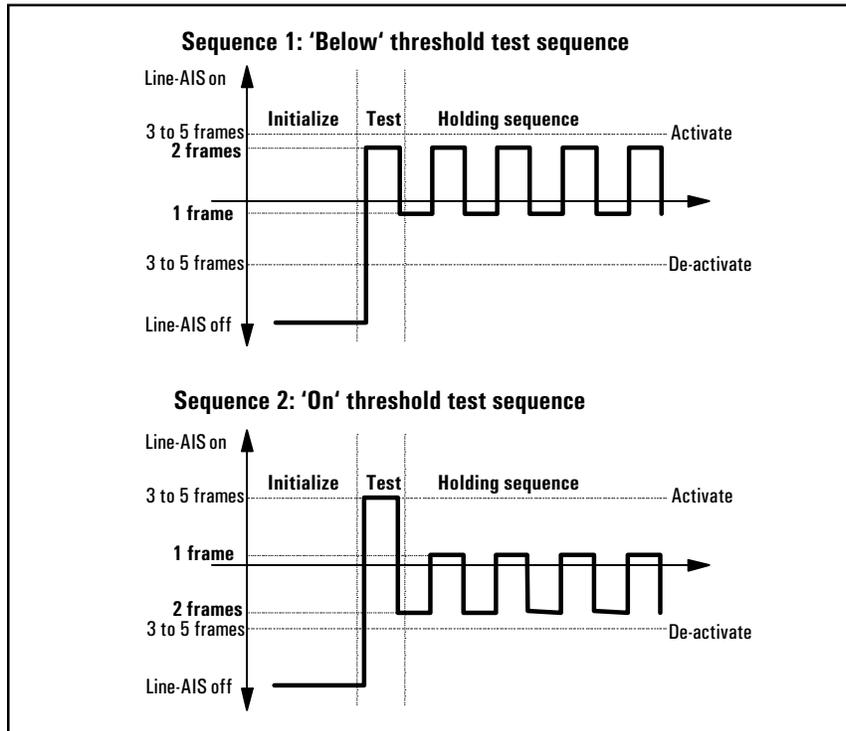
Figure 3. Line-AIS detection threshold test
