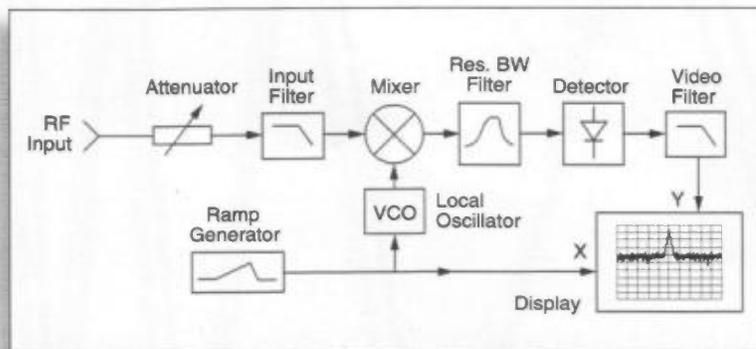
Figure 2. Spectrum analyzer block diagram.
