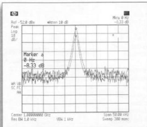
**Figure 1. Internally generated distortion products.**
