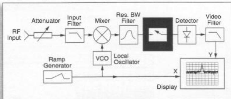
Figure 2. Spectrum analyzer block diagram with time gating.
