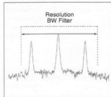
Figure 1. Resolution bandwidth setting.
