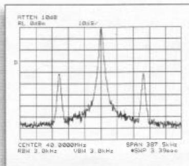
Figure 3. Spectrum with time gating.
