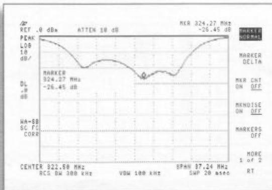
Figure 2. Return loss measurement.
