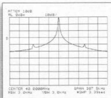
Figure 1. Spectrum without time gating.
