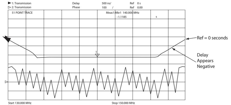
Figure 9. Filter measurement with insufficient number of points
