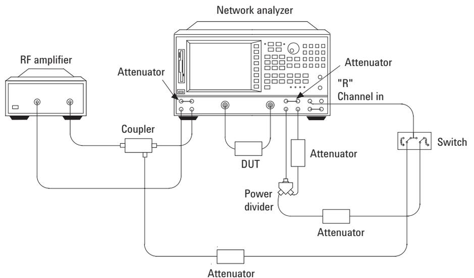
Figure 3. High-powered forward and reverse measurement configuration
