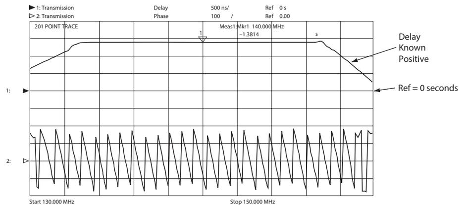
Figure 10. Filter measurement with correct number of points
