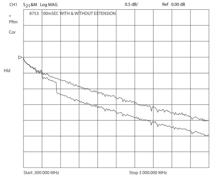
Figure 5. Reduce measurement error by balancing reference path
