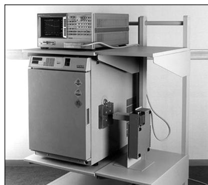
Figure 8. Using the Tabai Espec SU-240-Y temperature chamber with the 4291B
