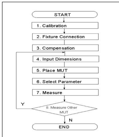
Figure 10. Magnetic material measurement process
