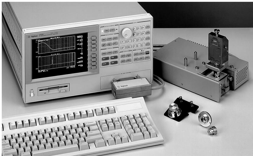
The Agilent 4291B RF impedance and material test system
