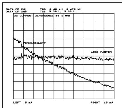
Figure 6. Relative permeability as a function of test current
