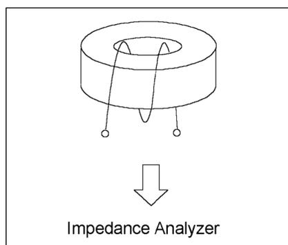
Figure 1. Hand-wound inductor method for permeability measurement
