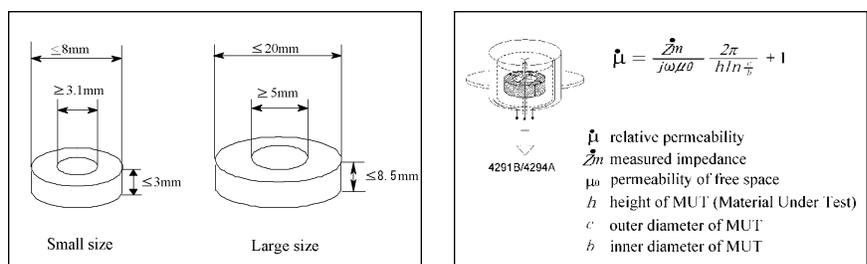
Figure 5. Inductor method permeability measurement
