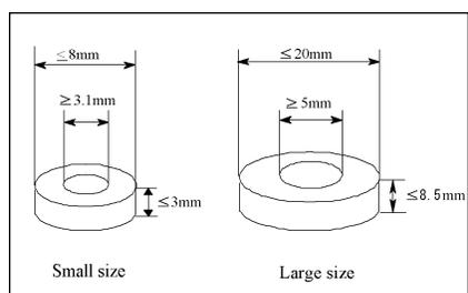
Figure 4. Toroid dimensions for the 16454A fixtures
