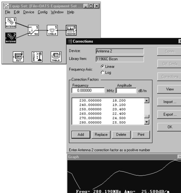
**Figure 24:** The 85876B can set up your equipment and import correction factors to correct for your measurement path.
