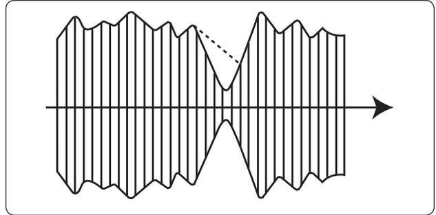
**Figure C. An envelope detector will follow the envelope of the shown signal, albeit with the delay and filtering action of the LPF used to remove the carrier harmonics. A peak detector is subject to negative slew limits, as demonstrated by the dashed line it will follow across a response pit. This drawing is done for the case in which the logarithmic amplification precedes the envelope detection, opposite to Figure A; in this case, the pits of the envelope are especially sharp.**
