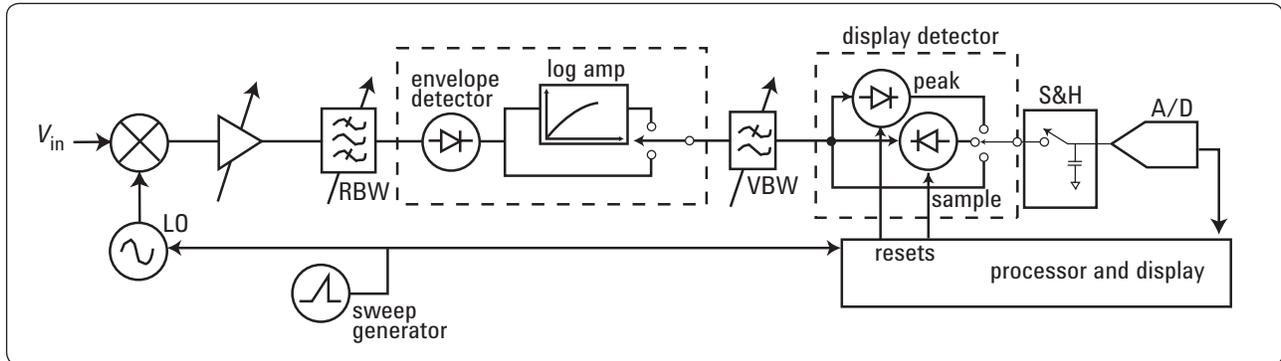
Figure A. Simplified spectrum analyzer block diagram
