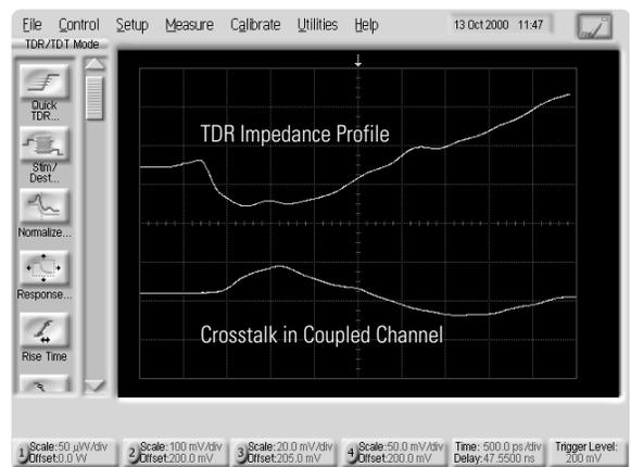
Figure 26. Crosstalk with lines unterminated (PGA)
