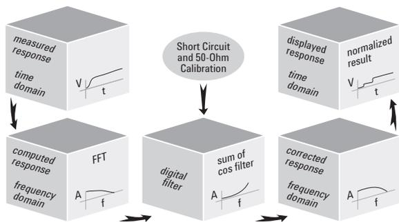
Figure 11. Normalization process
