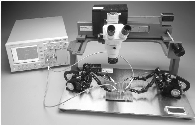
A guide to making accurate measurements with the Agilent 86100A Infiniium DCA and Time Domain Reflectometer using Cascade Microtech high frequency probes.
