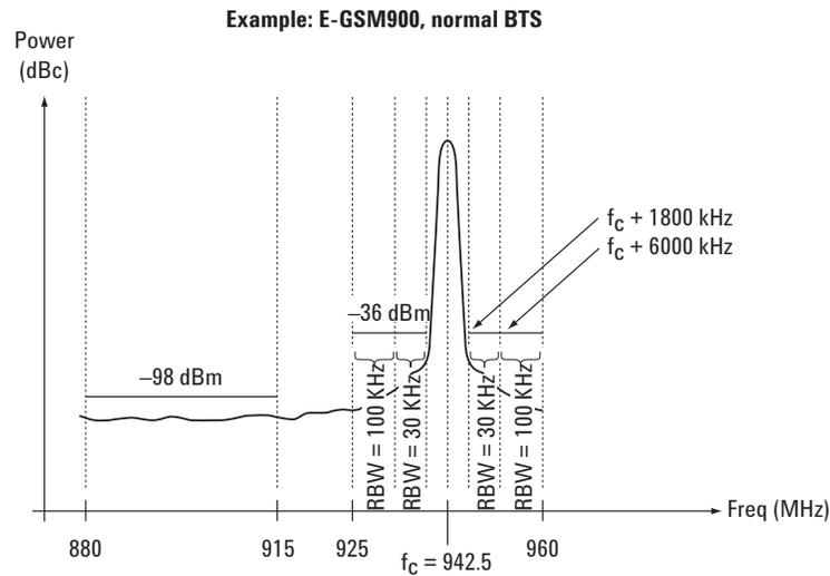
Figure 25. Tx and Rx band spurious, BTS, limits
