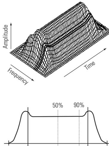
**Figure 18. Theory of spectrum due to modulation and wideband noise**
