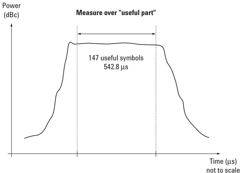
Figure 11. Theory of mean transmitted RF carrier power
