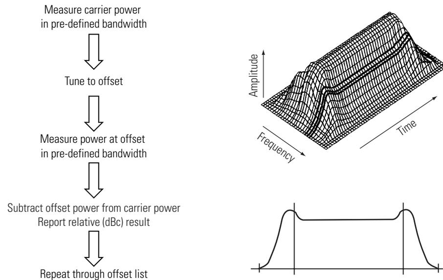
**Figure 21. Theory of spectrum due to switching**
