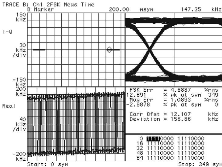
Figure 12. Agilent 89441A display of demodulation quality test
