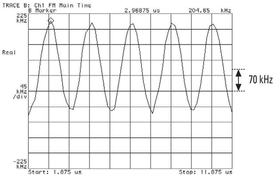
**Figure 13. Agilent 89441A display of initial carrier frequency tolerance measurement with a 70 kHz frequency offset**
