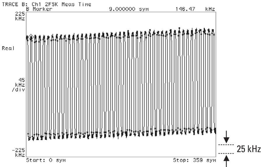
**Figure 14. Agilent 89441A display of carrier frequency drift measurement**
