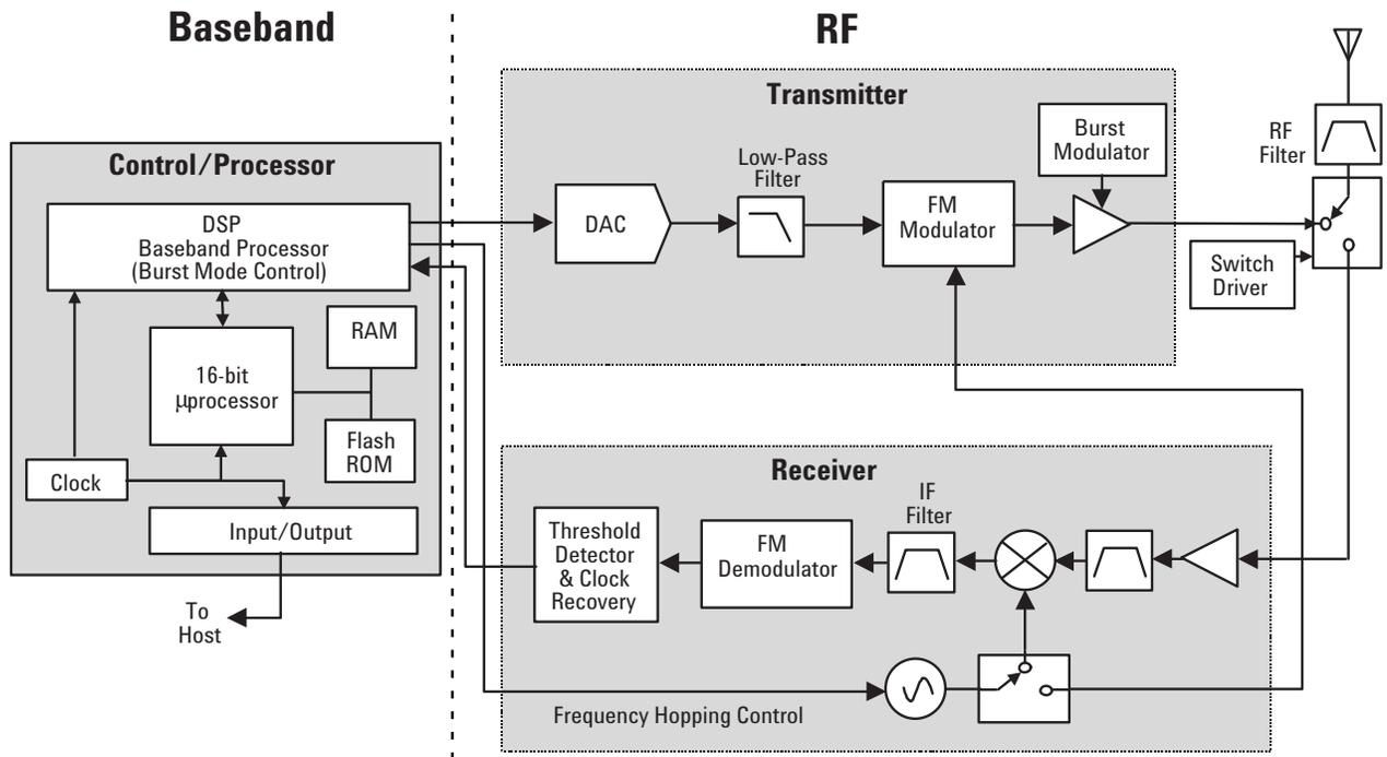
Figure 1. Block diagram of a Bluetooth system
