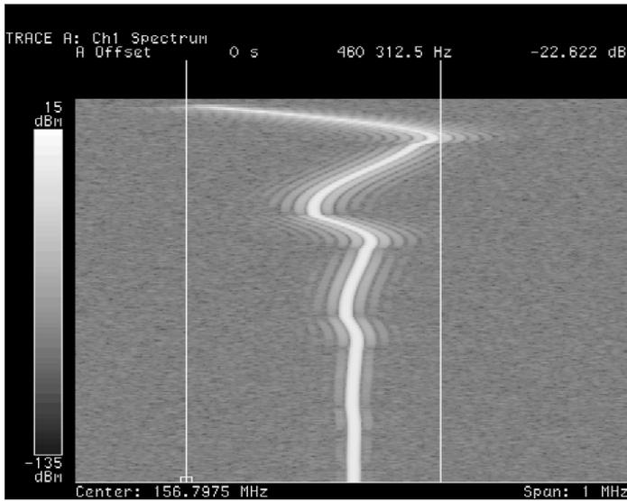
Figure 16. Agilent 89441A spectrogram display for PLL settling time
