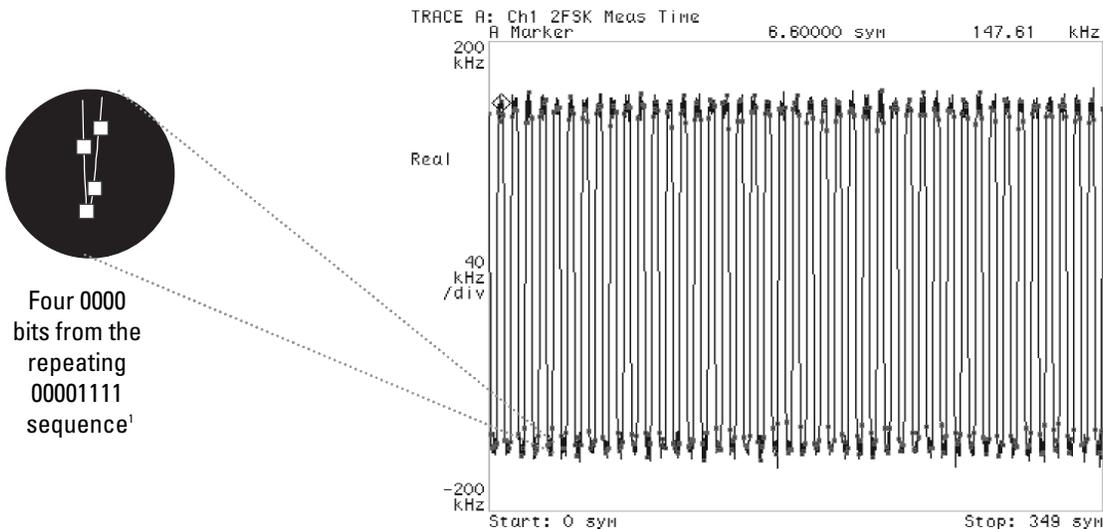
**Figure 11. Agilent 89441A display showing modulation characteristics measurement**
