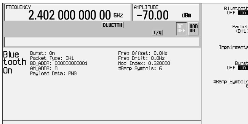
Figure 21. Agilent ESG-D series Option UND display of Bluetooth configuration menu
