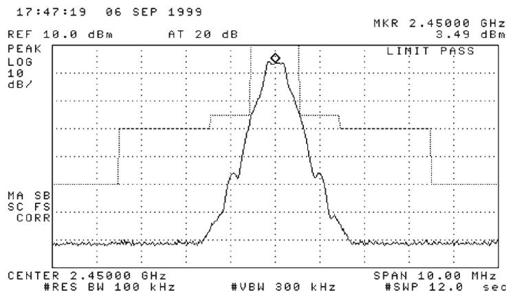
**Figure 10. Agilent 8594E display of output spectrum measurement (CF=2.45 GHz, Span=10 MHz, RBW=100 kHz, VBW=300 kHz, Sweep Time=12 s, Detector Sample Mode, Trace Max Hold, Limit Line Mask)**
