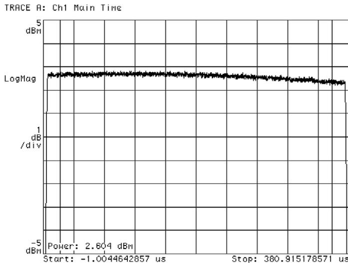
**Figure 8. Agilent 89441A display of average and peak power measurement**
