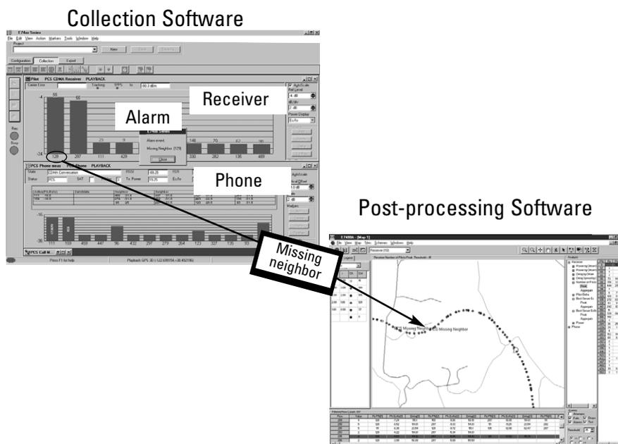
**Figure 22. Integrated drive-test solution with RF receiver and phone quickly identifies "missing neighbor" condition. Alarms and post-processing software simplify the identification of wireless network problems.**
