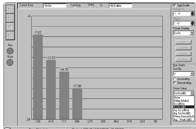
**Figure 15.** Receiver Top N pilot measurement window.
