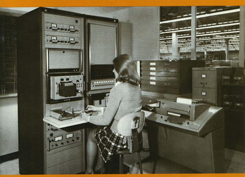
An IC test in progress on the Hewlett-Packard 9500 Automatic Test System.
