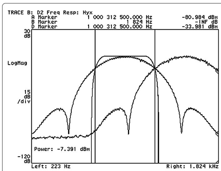
**Figure 12. The nearly-centered trace is the first proposed measurement filter, a 90 kHz single-sided bandwidth (180 kHz DSB) raised-cosine filter with an alpha of 0.25. The EDGE symbol rate is 270.833kHz, which is greater than the bandwidth of the measurement filter!**
