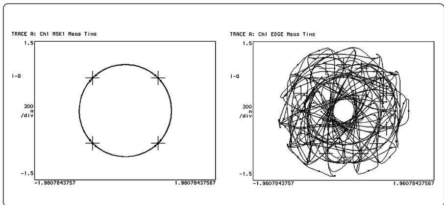
**Figure 2. The GSM signal on the left has a constant power envelope, unlike the EDGE signal at right. The plot represents the carrier magnitude and phase at any given point in time. Since the carrier amplitude for GSM is constant, the carrier trajectory forms a perfect circle.**
