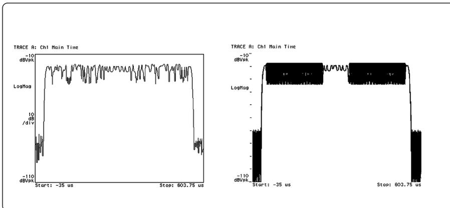
**Figure 4.** The power vs. time plot at left shows a single EDGE burst, while several hundred bursts are overlaid in the plot at right.
