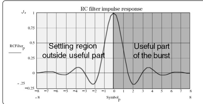
**Figure 13. The first proposed 0.25 alpha, raised-cosine filter’s impulse response has the potential to introduce errors into the useful part of the signal burst from the settling region, or even from adjacent time slots!**
