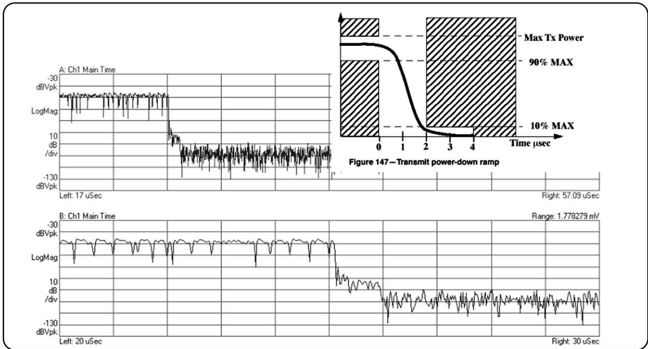
Figure 2.3.6: 802.11b power-down-envelope mask
