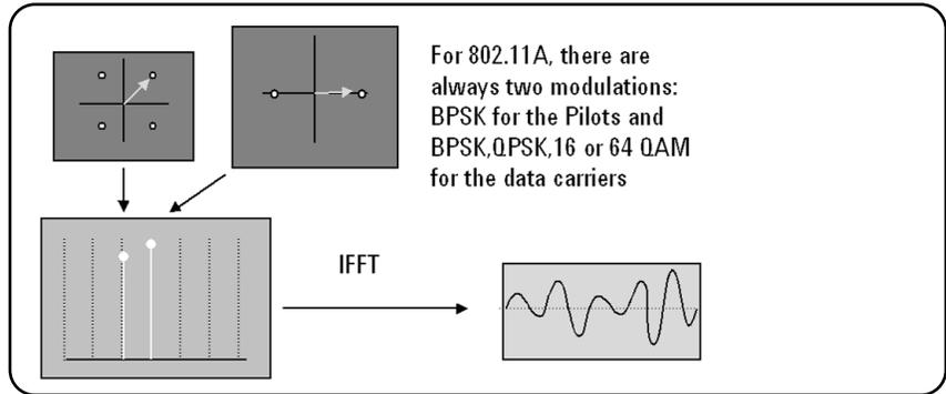
Figure 3.1.7: IFFT used to create multiple carriers
