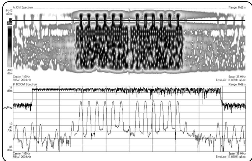
Figure 3.3.6: Spectrogram analysis of an OFDM burst
