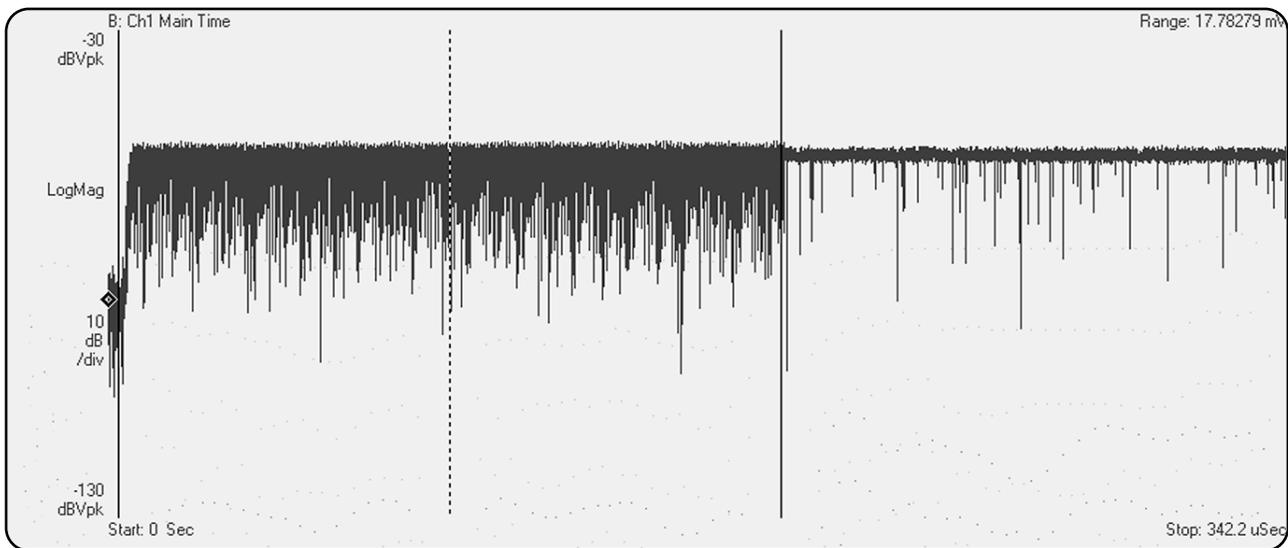
Figure 2.3.2: 802.11b burst with longer data segment
