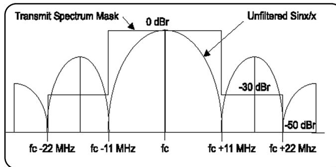
Figure 2.3.7: 802.11b transmit spectral mask
