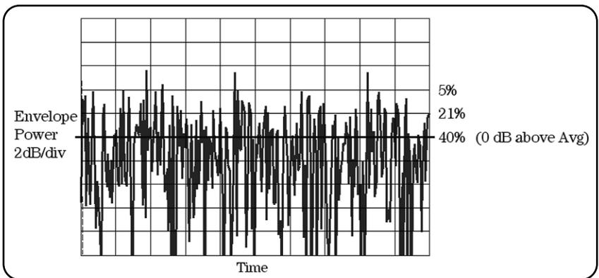
Figure 3.3.8: Power versus time for an OFDM burst
