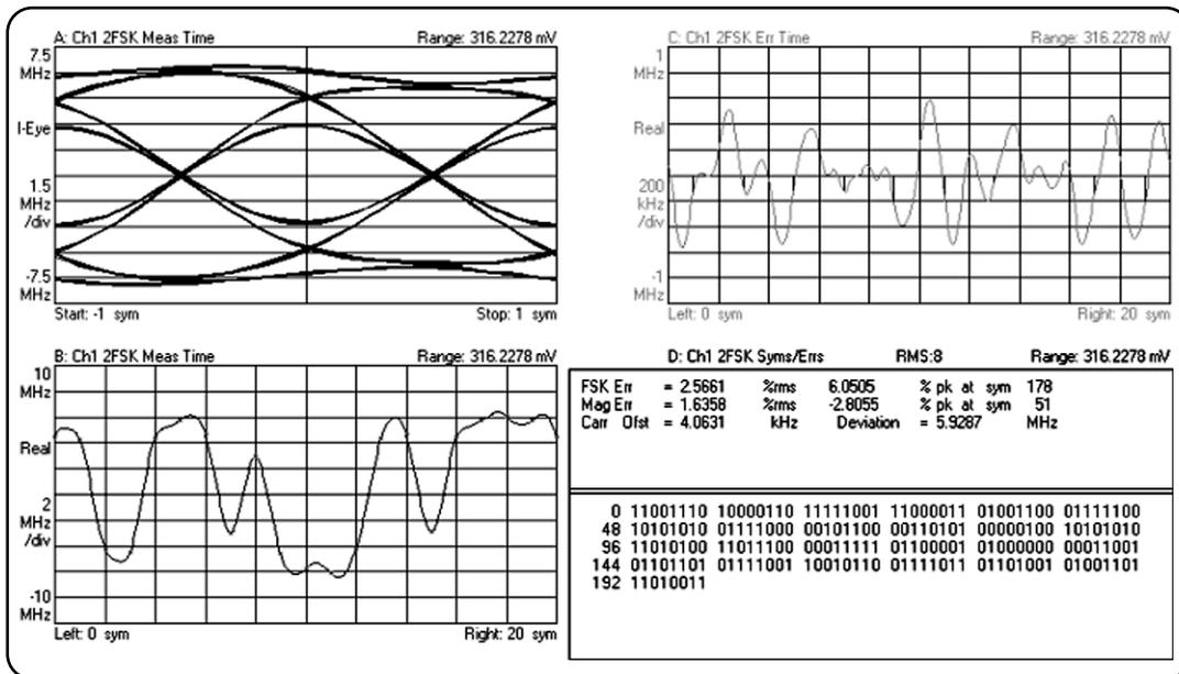
Figure 1.3.2: GMSK signal demodulated as a GFSK signal
