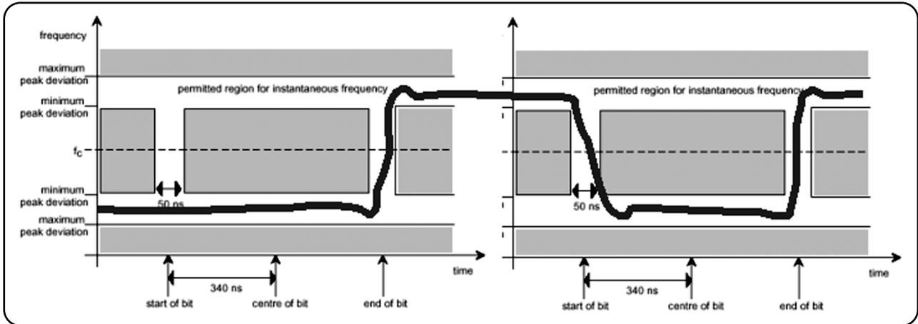
Figure 1.1.2: Eye-diagram mask for low-rate FSK modulation
