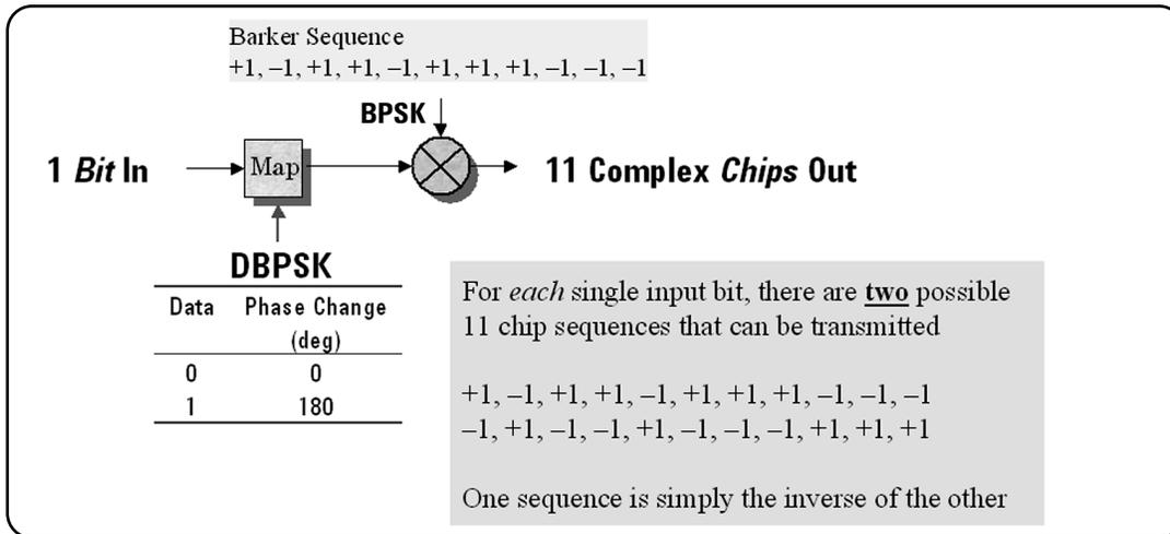
Figure 2.1.1: DSSS signal spreading for 1 Mbit/sec data rate
