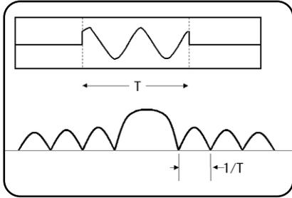
Figure 3.1.4: Spectral shape of a signal OFDM carrier
