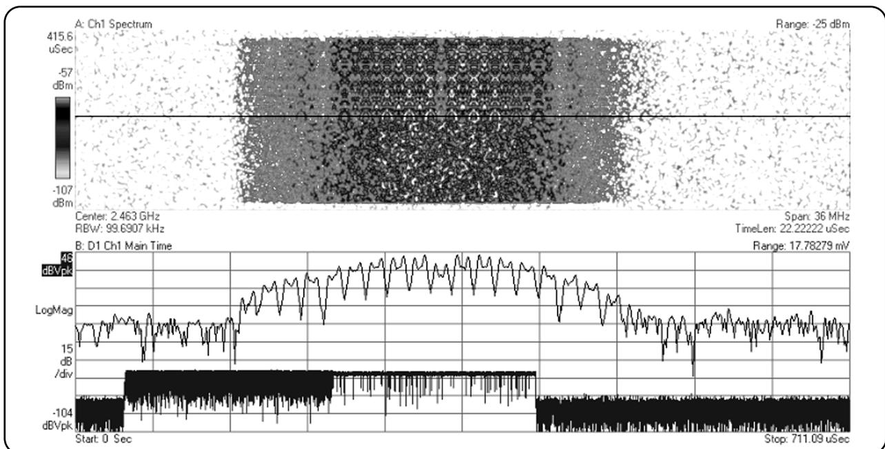
Figure 2.3.9: Spectrogram analysis of a single 802.11b burst
