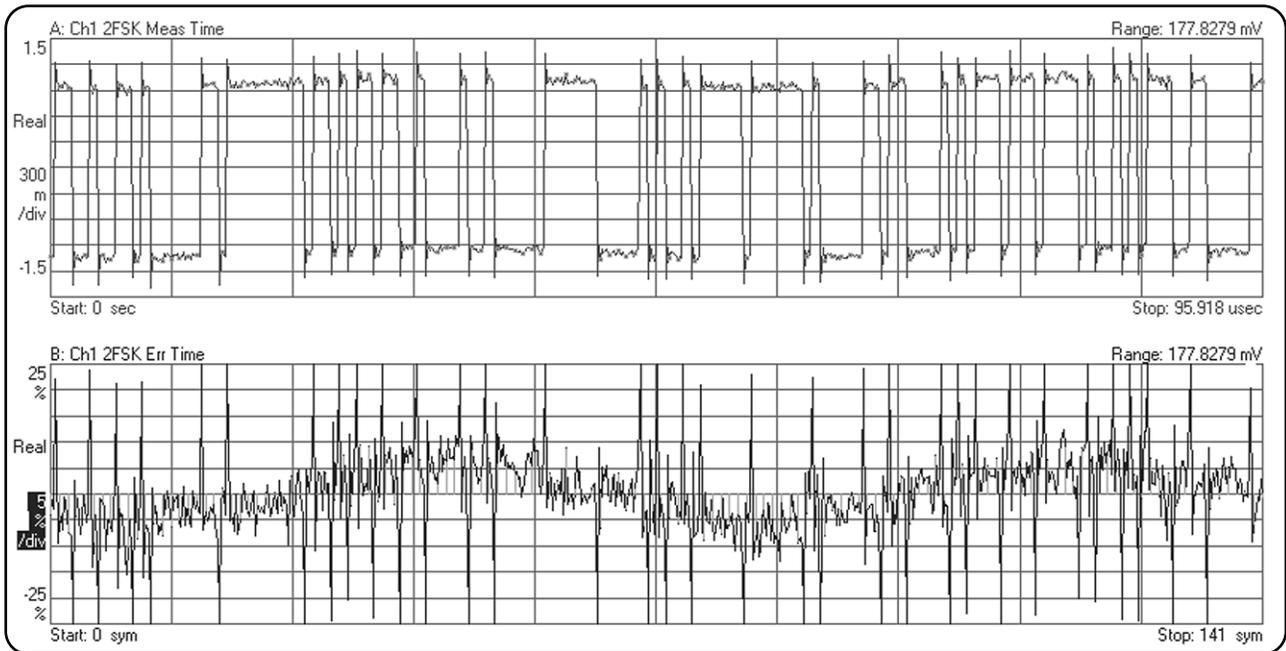
**Figure 1.1.3: Residual FM on a FSK waveform**
