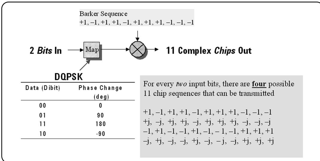
Figure 2.1.2: DSSS signal spreading for 2 Mbit/sec data rate
