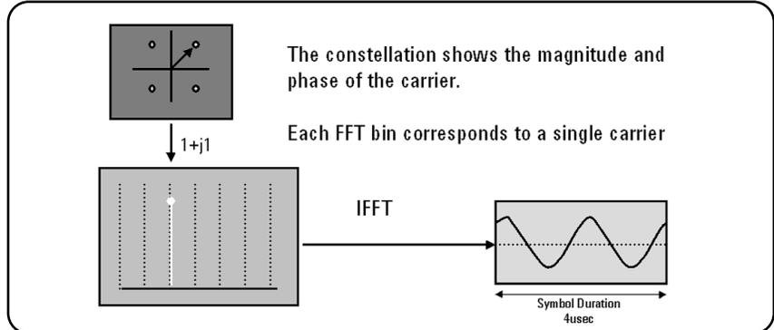
Figure 3.1.5: IFFT used to create one carrier
