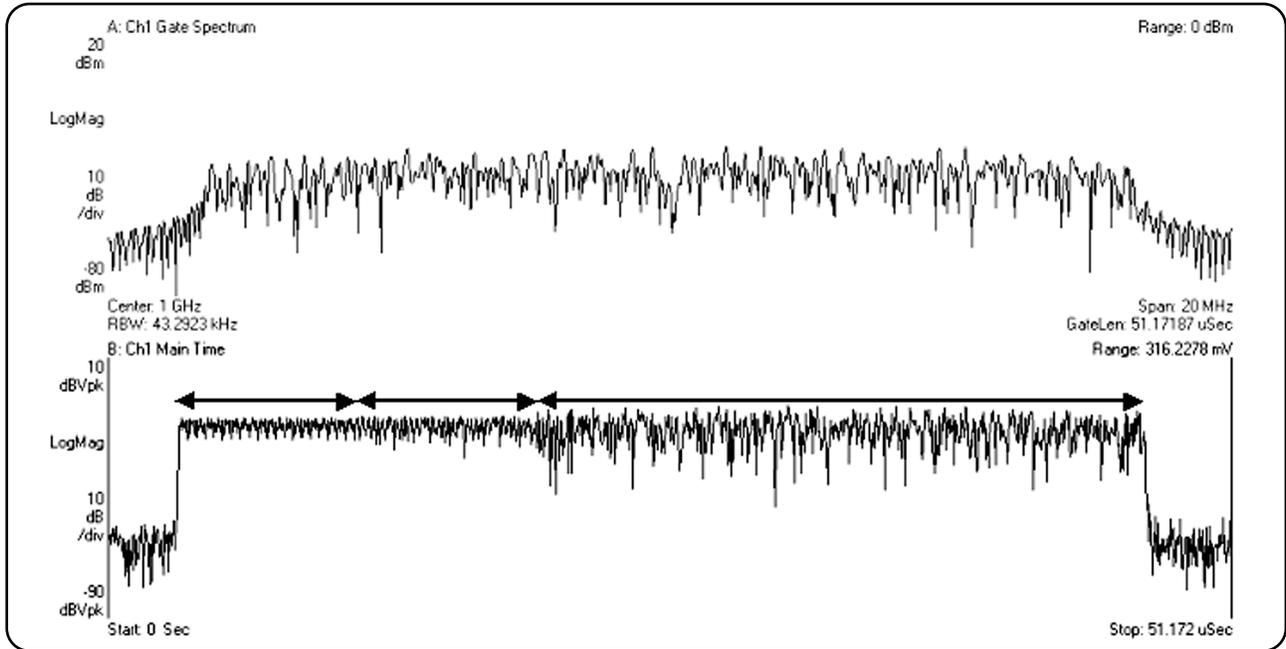
Figure 3.3.1: OFDM power burst and spectrum
