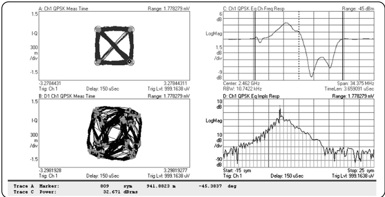
Figure 2.3.14: Effects of equalization on signal demodulation
