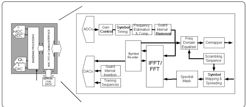
Figure 3: Digital processing blocks for an OFDM transceiver
