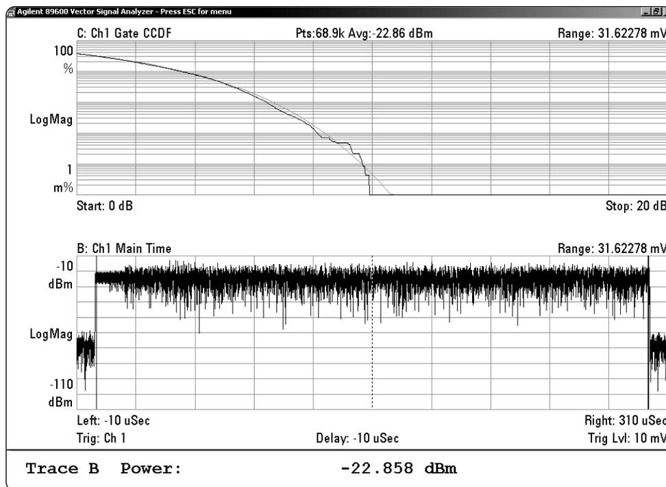
**Note:** Measurement gating must be used to avoid including a zero power reading between bursts.
