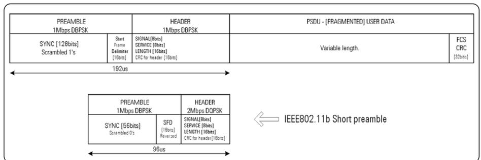
Figure 5: IEEE 802.11b frame structure with short/long sync
