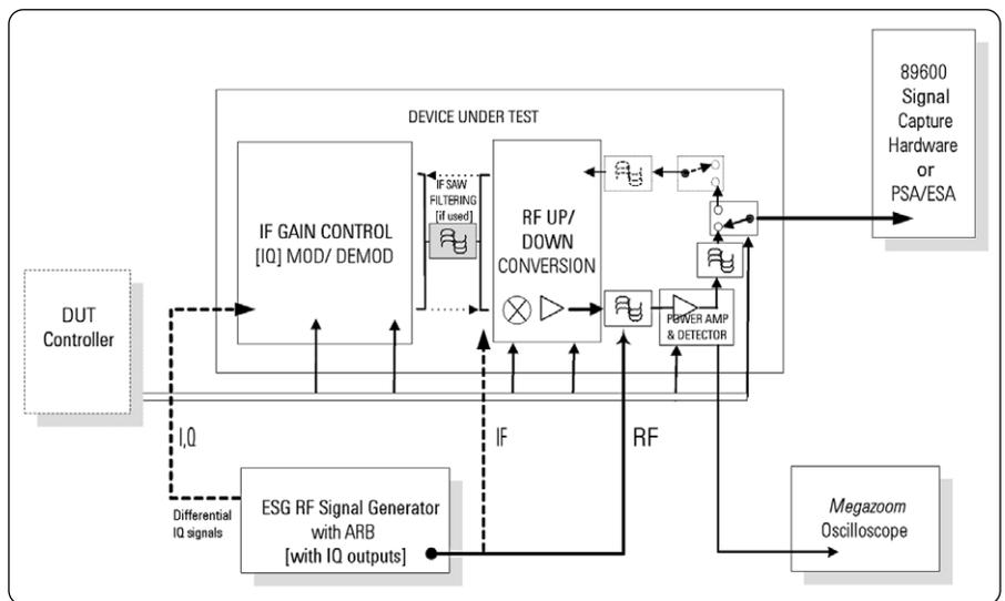
Figure 7: Transmitter test configuration for RF/analog circuitry
