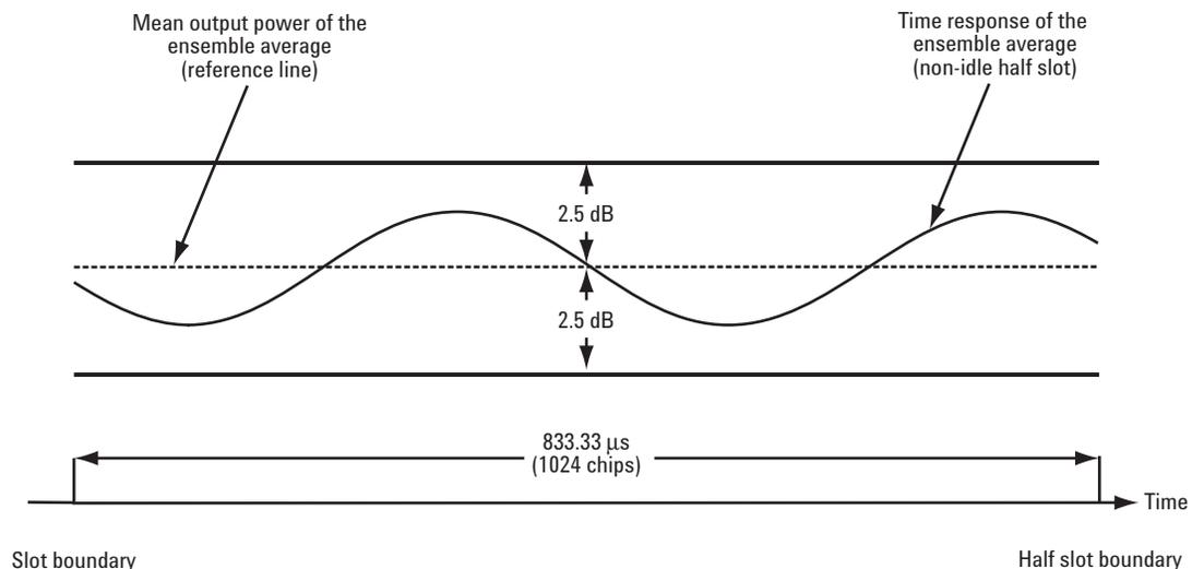
Figure 8. Transmission envelope mask of average active half-slot
