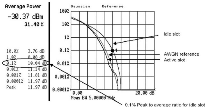
Figure 13. CCDF curves for an active slot (QPSK) and an idle slot (pilot only)
