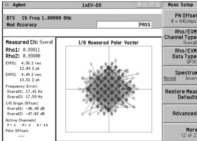
**Figure 19. Modulation accuracy of composite forward link**
