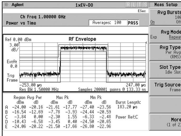
Figure 10. Power versus time measurement
