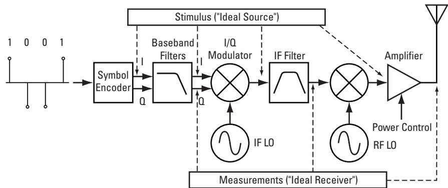
Figure 7. Transmitter chain measurement model
