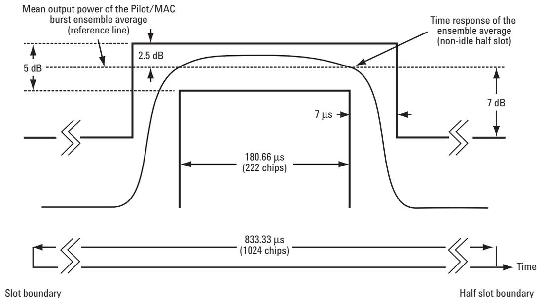
Figure 9. Transmission envelope mask for average idle half-slot
