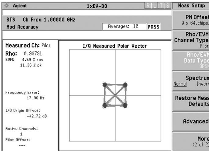
Figure 17. Modulation accuracy of pilot channel
