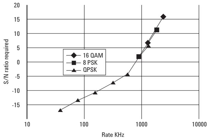
**Figure 3. S/N versus data rate**
