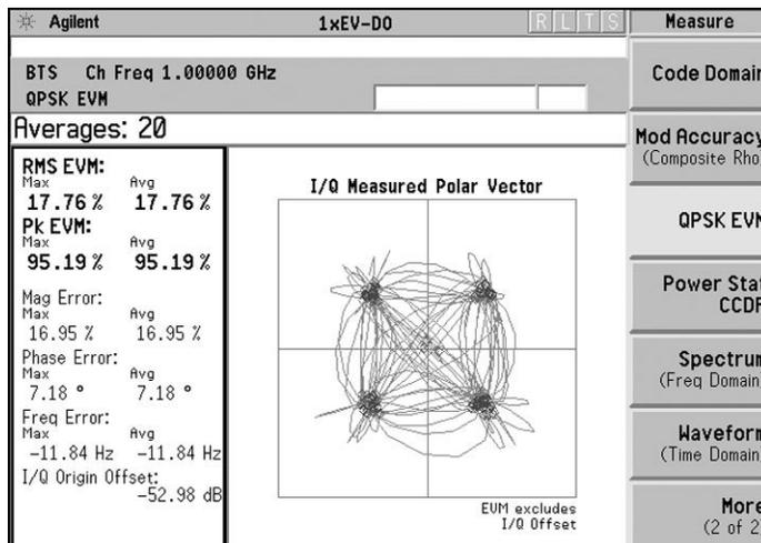
**Figure 23. QPSK EVM measurement results**
