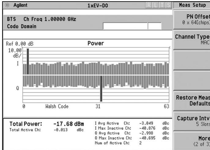
Figure 21. Code domain measurement with two MAC channels active
