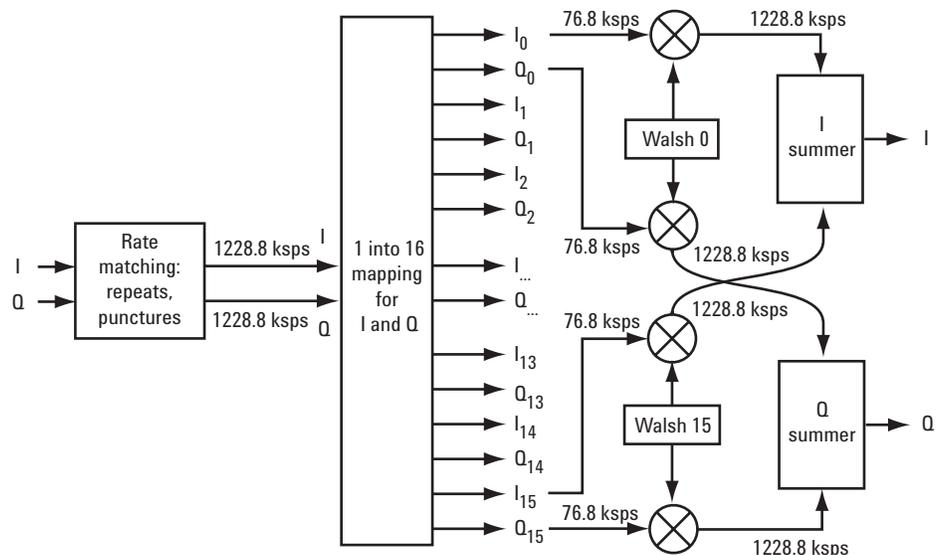
**Figure 5. Rate matching and Walsh encoding**
