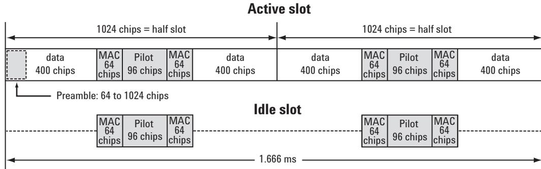
**Figure 2. TDM structure for 1xEV-DO active and idle slots**
