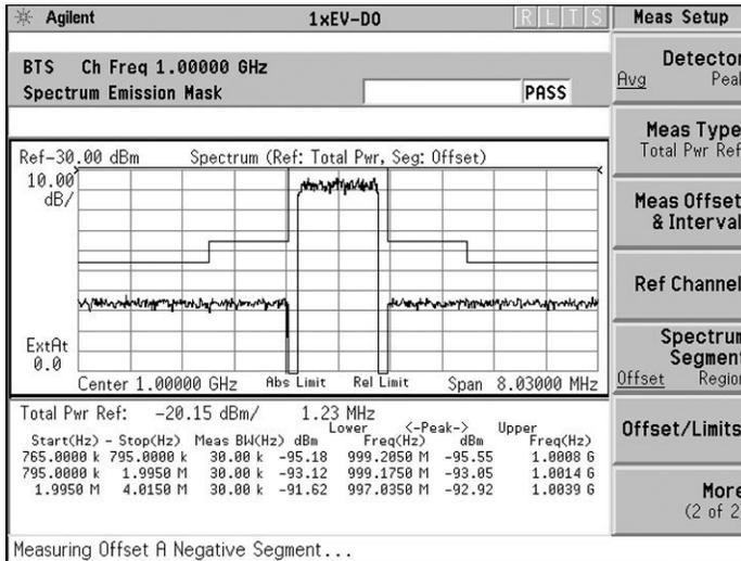
**Figure 11. SEM measurement for idle mode**
