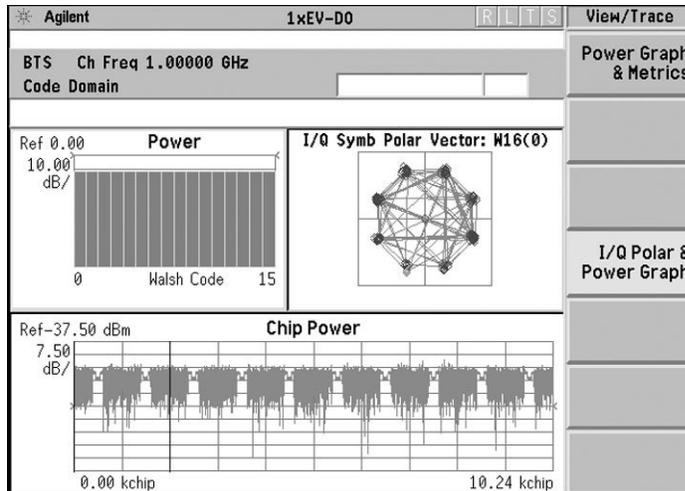
**Figure 22. Code domain measurement with traffic channels active with 8PSK modulation**
