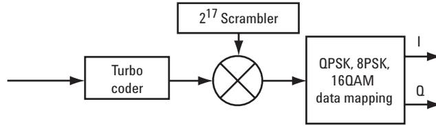
**Figure 4. Traffic channel coding for the forward link**
