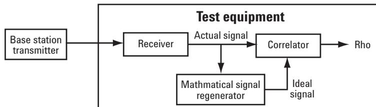
Figure 16. Typical rho measurement setup
