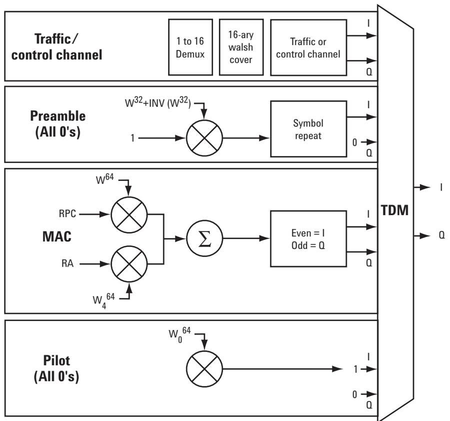
Figure 1. TDM structure of the 1xEV-DO forward link
