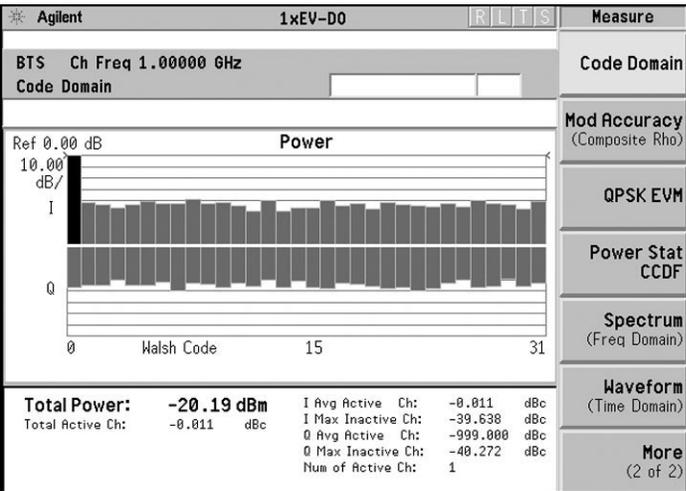
Figure 20. Code domain measurement with only pilot active
