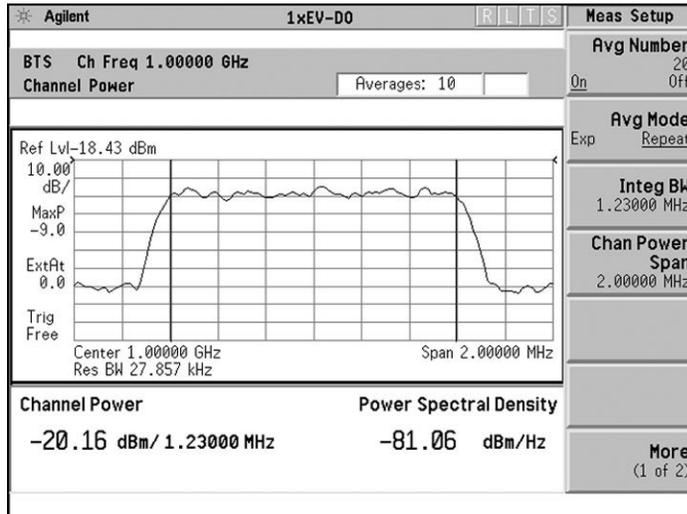
Figure 15. Channel power measurement
