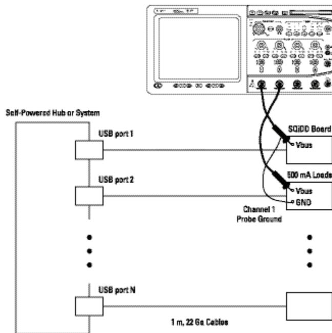
Figure 8. Droop setup for hosts and self-powered hubs.
