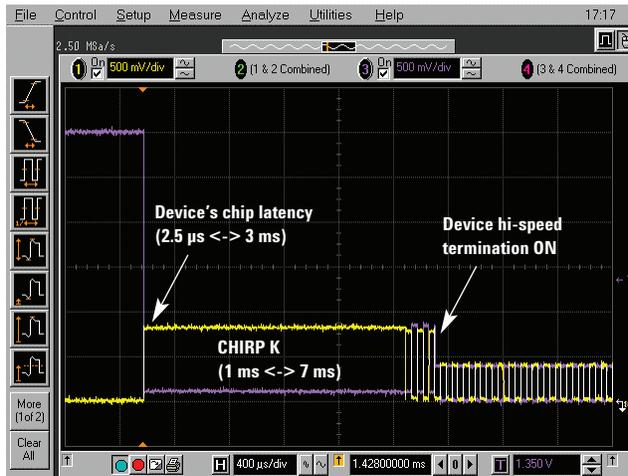
Figure 15. CHIRP test.
