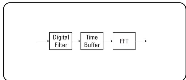
Figure 8.2. Time buffer added to block diagram
