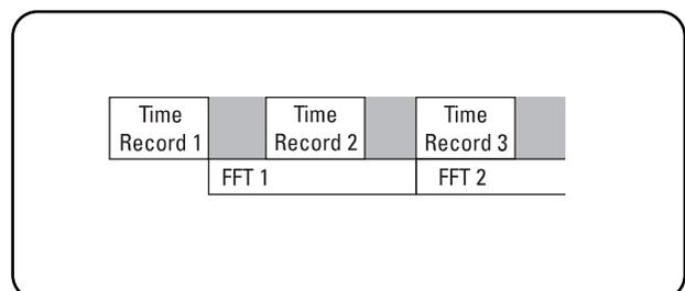
Figure 8.4. Non-real-time operation
