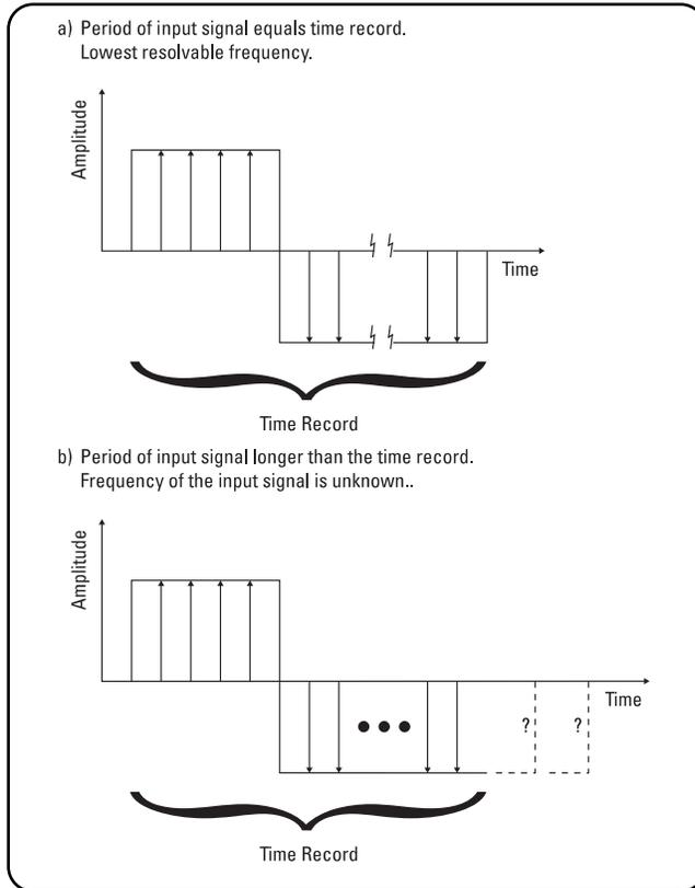
Figure 1.7. Lowest frequency resolvable by the FFT
