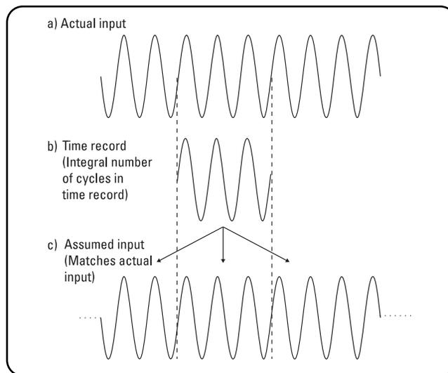
Figure 5.2. Input signal periodic in time record
