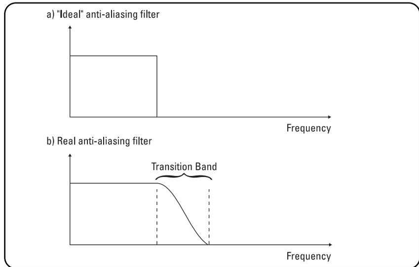
Figure 3.7. Actual anti-alias filters require higher sampling frequencies.
