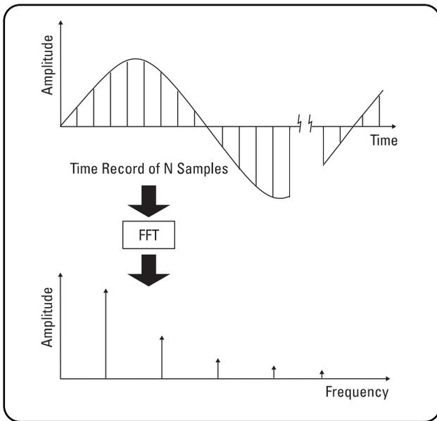
Figure 1.3. The FFT works on blocks of data.
