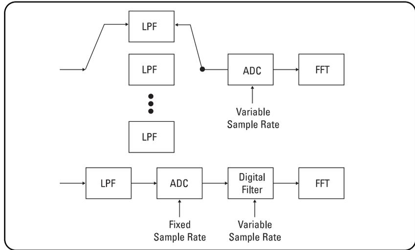
Figure 3.8. Block diagrams of analog and digital filtering
