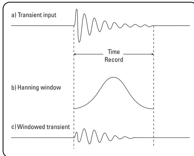
Figure 5.8. Windowing loses information from transient events.
