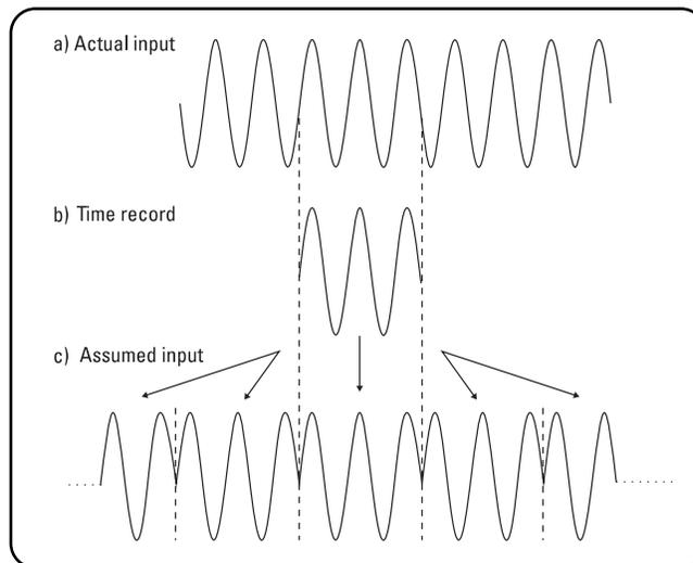
Figure 5.3. Input signal not periodic in time record
