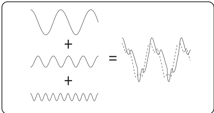
Figure 1.6. Phase of frequency domain components is important.
