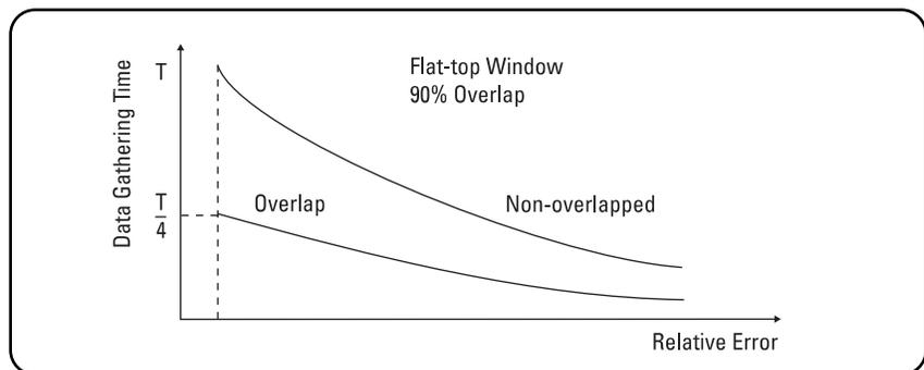
Figure 9.2. RMS averaging speed improvements with overlap processing
