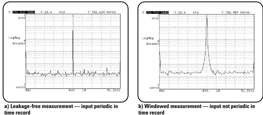
Figure 5.7. Windowing reduces leakage but does not eliminate it.
