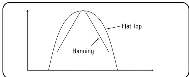
Figure 5.13. Reduced resolution of the flat-top window
