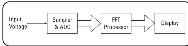
Figure 2.1. Block diagram of a dynamic signal analyzer
