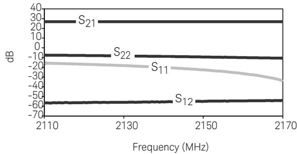
Figure 9. DUT S-parameters, with and without pre-amplifier
