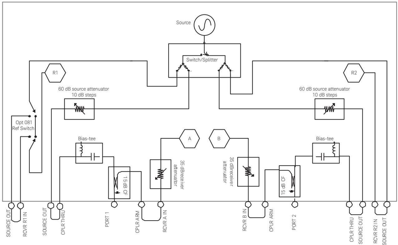
Figure 1. PNA (E8362/3/4B) block diagram for basic measurements
