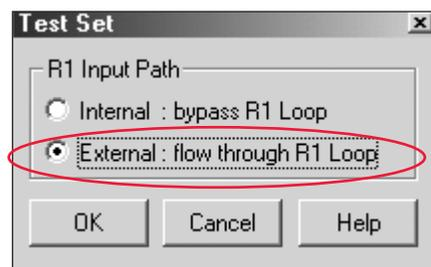
1. Option 081, External Reference Switch, is used primarily for mixer and converter measurements and is not required for amplifier measurements. However, if your analyzer is equipped with Option 081, you need to set the position of the external reference switch.
