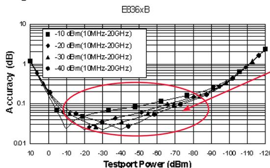
For best measurement accuracy, select the measurement and calibration power levels such that the test setup power levels remain in the relatively flat region.
