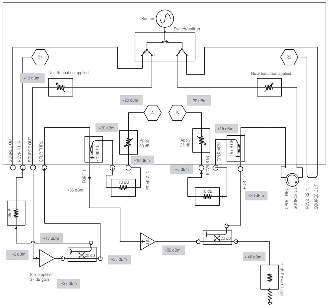
Figure 4. MW PNA E8362B-H85, configured to measure a solid state power amplifier
