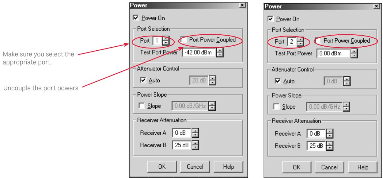
In order to determine the power levels at each port, go through the block diagram and perform the various calculations. In step A, linear testing, the power incident upon our amplifier was -10 dBm. The goal here is to determine the various settings in order to once again achieve -10 dBm at the amplifier input.
