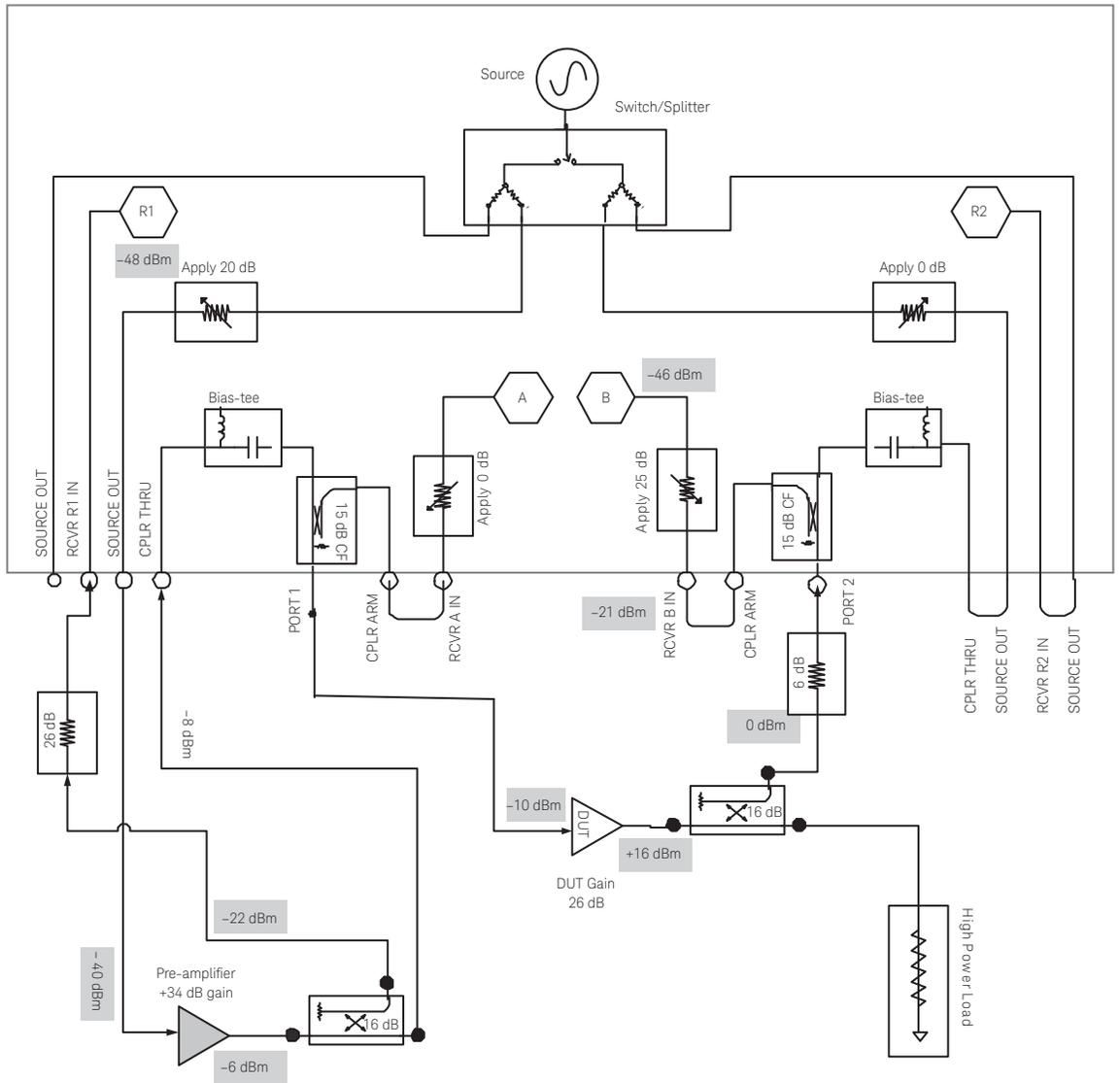
Figure 8. High-power setup, for low-power testing of S-parameters
