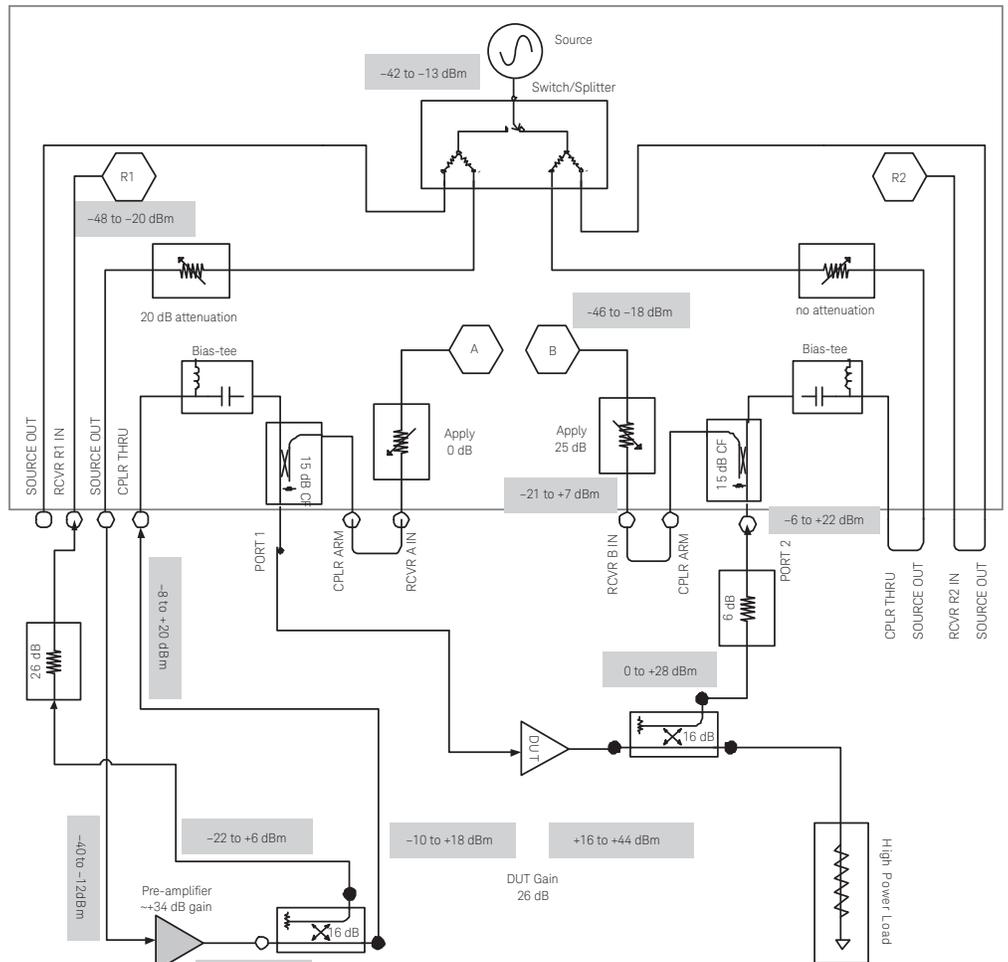
Figure 11. A power sweep for gain compression test.
