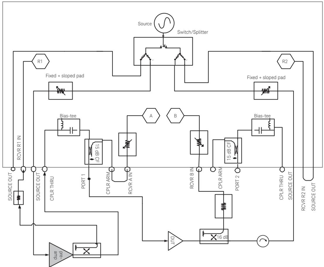
Figure 13. Use of external coupler in high-power measurements
