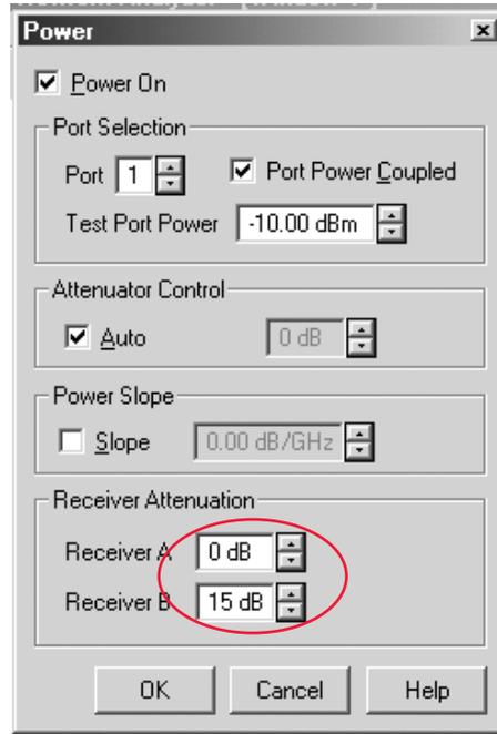
Slowly increase the power level and observe the gain; it should not change until you approach the compression of the amplifier under test. However, we cannot compress this amplifier with the power directly available from the PNA.
