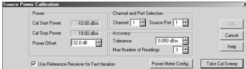
Next we perform a response calibration for the  $S_{21}$  measurement. For the absolute B receiver measurement, we perform a source and receiver calibration. The gain compression of the amplifier under test is shown in Figure 12
