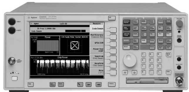
Agilent PSA high performance spectrum analyzer with the 1xEV-DO measurement personality
