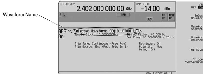
Figure 38. ESG dual arbitrary waveform generator user interface.
