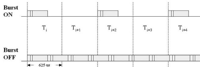
Figure 16. Bursted and non-bursted single slot packet transmission.
