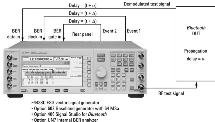
**Figure 18.** To perform BER analysis using this measurement setup, the clock/gate delay setting ( $\Delta$ ) must be equal to the propagation delay the test signal experiences through the *Bluetooth* device ( $\alpha$ ).
