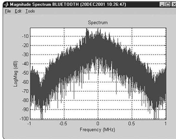
Figure 37. Spectrum plot of the *Bluetooth* I/Q waveform.
