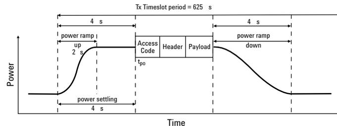
**Figure 15. Burst profile of a single slot packet transmission with 2  $\mu$ s power ramp and 4  $\mu$ s ramp settling.**
