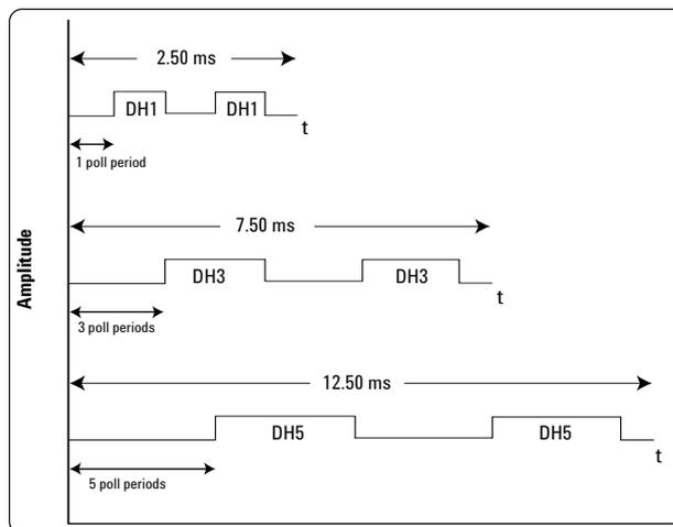
Figure 28. Timing diagram for test set for each packet type. ~~Use with External Frame Sync~~ is selected, the DH1 impairment set consists of four packets.
