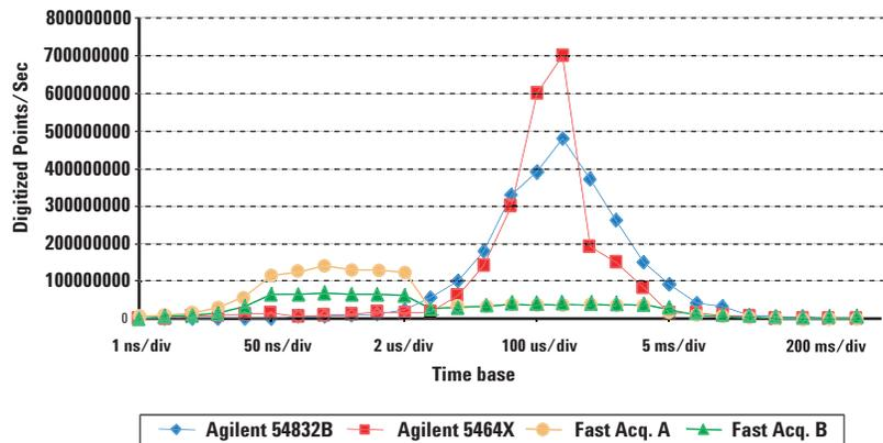
Note: Measurement conditions: Realtime sampling, 1 channel acquisition, sinx/x interpolation OFF, markers OFF, math OFF, connect dots ON, stats OFF, sinewave input with ~5 cycles per screen, number of digitized points based on "on-screen" viewable points only.
