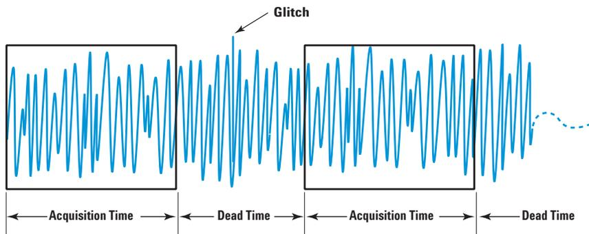
Figure 1. Digitizing oscilloscope acquisition time versus dead time
