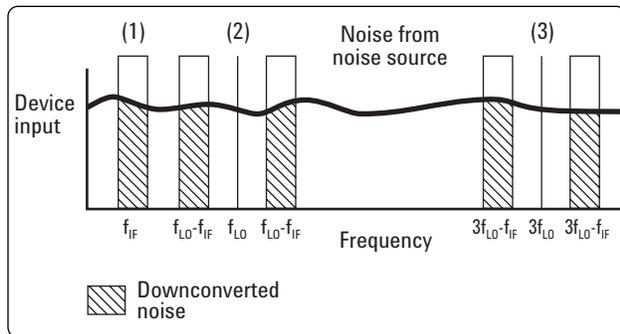
Figure 2.4. Possible noise conversion mechanisms with mixers and converters. (1) IF feedthrough response, (2) double sideband response, (3) harmonic response
