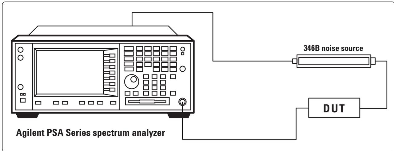
Figure 1.1. The PSA Series Option E444xA-219 Noise Figure Measurement Personality operates in the measurement system shown here. The spectrum analyzer is used as the measurement receiver, and also provides bias power to switch the noise source on and off during measurements.
