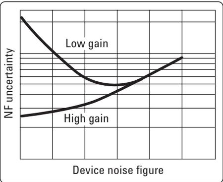
Figure 4.2. The uncertainty versus device noise figure curve
