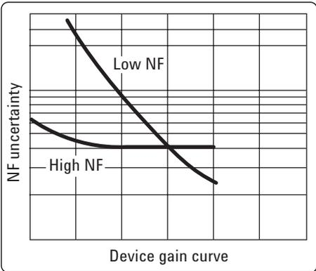
Figure 4.1 The uncertainty versus device gain curve
