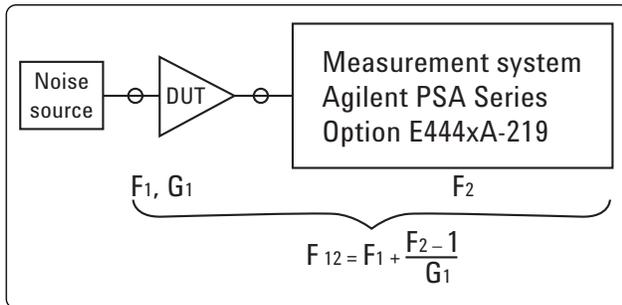
Figure 3.1. Typical noise figure measurement setup. Device and measurement system noise figures combine according to the cascade noise figure equation.
