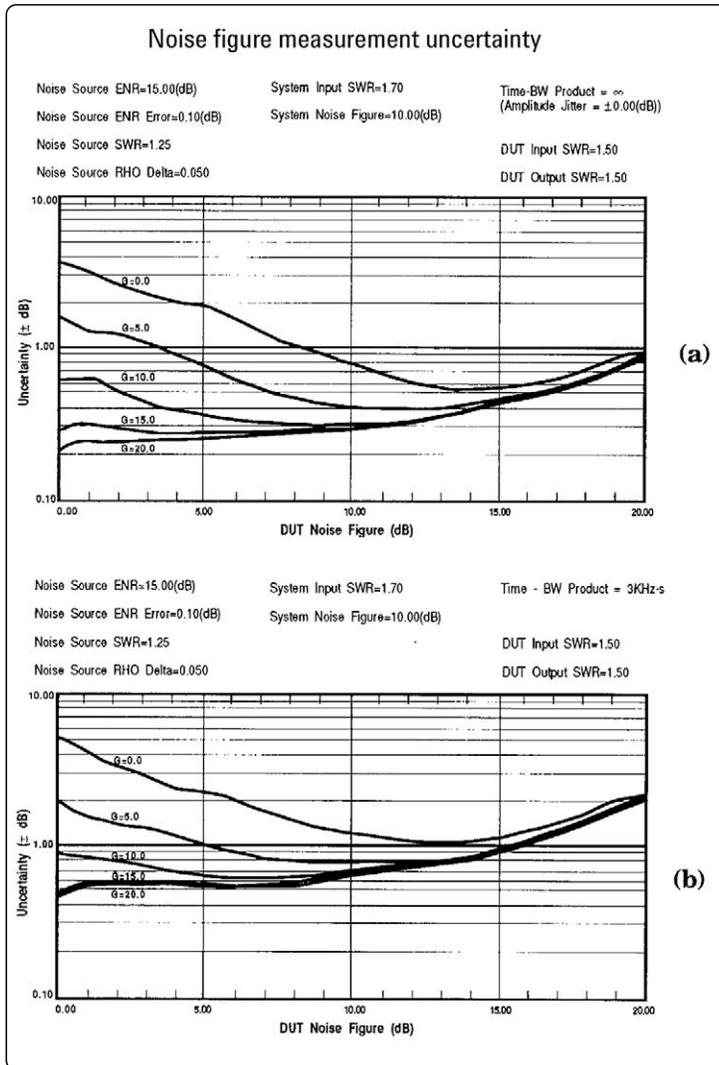
Figure 4.5. Effect of jitter on measurement error, (a) without jitter and (b) with jitter.
