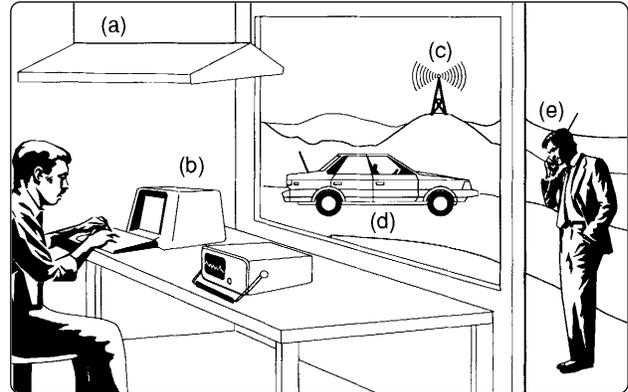
Figure 2.1. Signals can get coupled into a noise figure measurement from many different sources (a) fluorescent lights (b) computers and other instruments (c) local tv/radio stations (d) mobile radio (e) portable two-way radio or phone.
