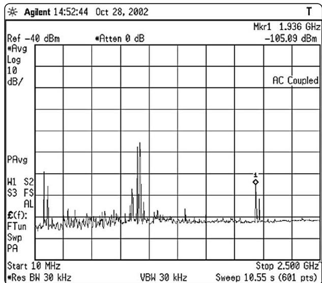
Figure 2.2. Stray signals can be found and measured directly using PSA in its normal spectrum analyzer mode. The built-in preamplifier (Option E444xA-1DS) can be used to make these measurements faster and more accurate.
