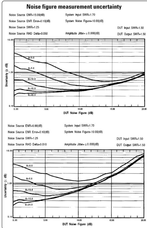
Figure 2.3. The effect of the noise source ENR on noise figure measurement uncertainty
