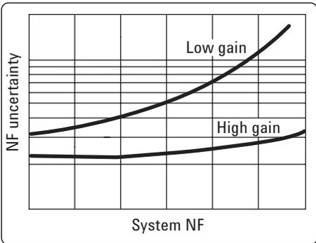
Figure 4.3. The uncertainty versus the system noise figure curve
