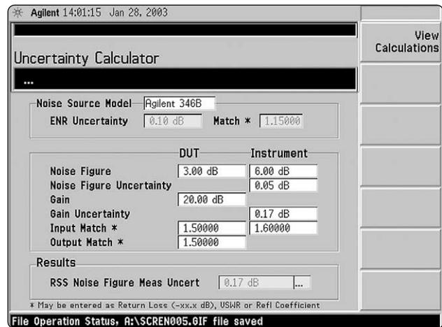
Figure 5.1. Internal measurement uncertainty calculator for the PSA Series Option E444xA-219
