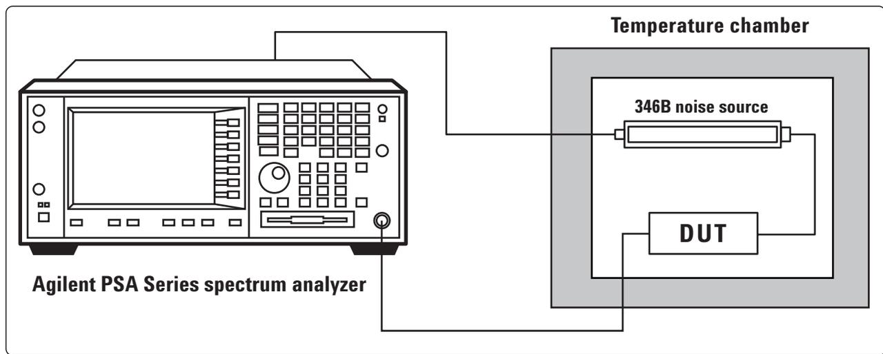
Figure 2.5. Temperature chamber with device under test and noise source inside
