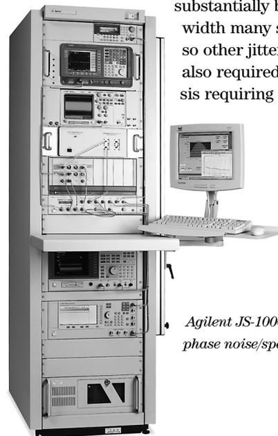
*Agilent JS-1000 low-level, phase noise/spectrum analyzer*
