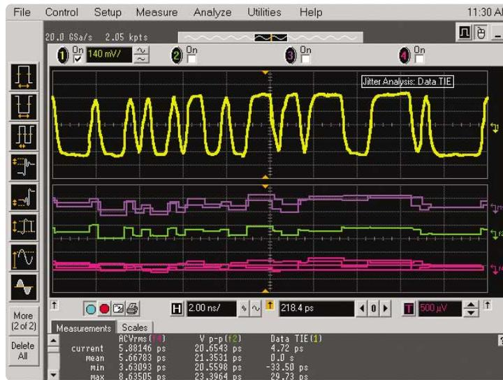
Figure 17. Measuring system Random Jitter (RJ).
