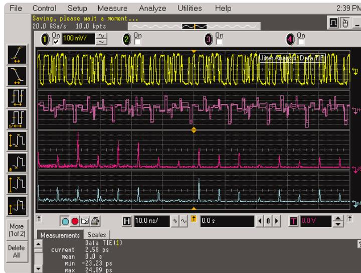
**Figure 16. Detecting correlated Periodic Jitter (PJ).**
