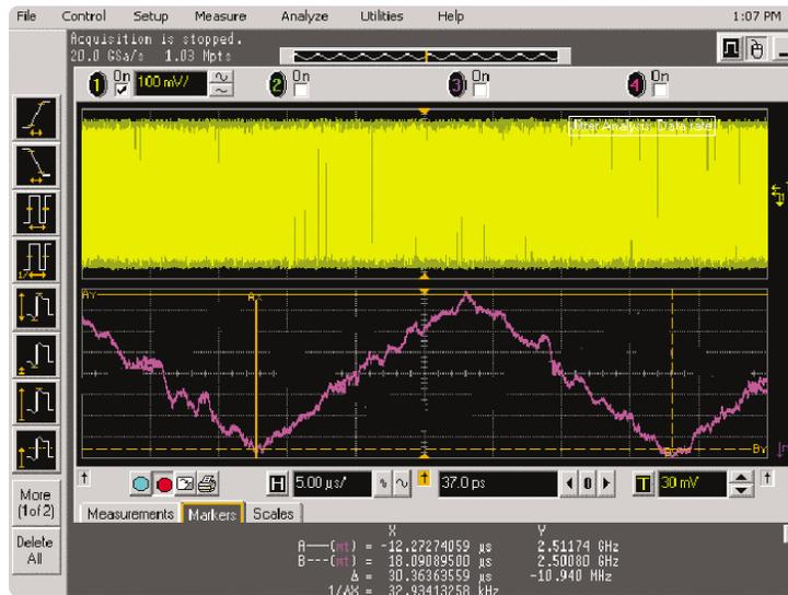
Figure 18. Measuring the Spread Spectrum Clock.
