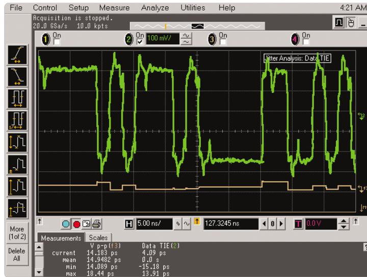
Figure 13. Testing for reflections at the transmitter side.
