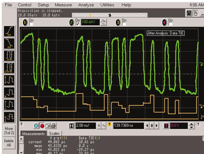
Figure 11. Isolating Inter-symbol Interference (ISI).
