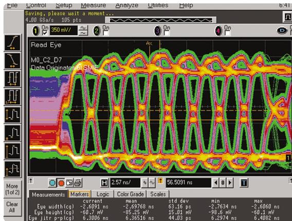
Using the control signals for the trigger, as seen at the top of Figure 3, he was able to observe bit D0 with an analog scope channel, and exclusively on “reads.” A standard four channel scope could not have been able to qualify this capture.
