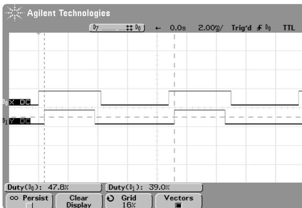
Figure 2b. Y-axis sensitivity (Min and Max duty cycles, X at 0 g)
