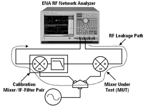
Figure 2. RF leakage path that would result in measurement errors
