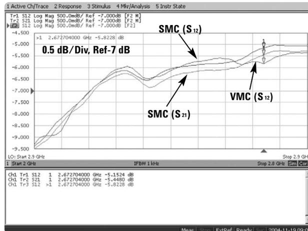
Figure 3. Conversion loss measurement comparison (SMC vs. VMC)
