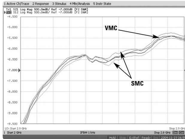
**Figure 7. Conversion loss measurement results with isolators**
