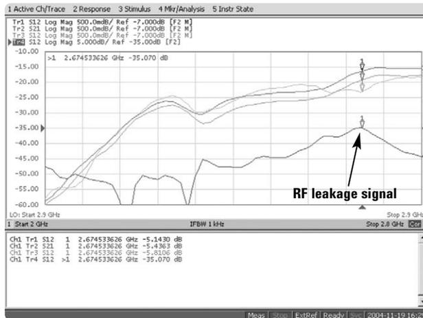
Figure 5. RF leakage through the LO port
