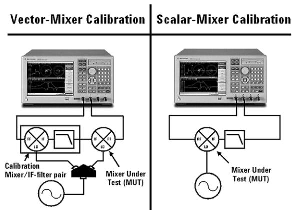
**Figure 1. Configurations of vector- and scalar-mixer calibration**
