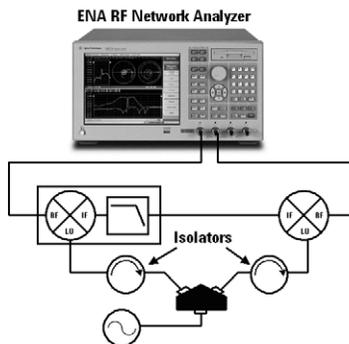
**Figure 6. Increase the measurement accuracy by using isolators in key positions**
