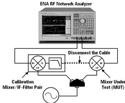
Figure 4. Verify the RF leakage
