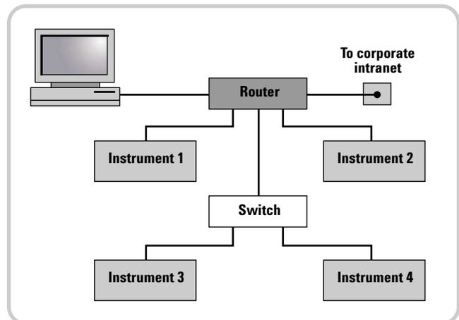
**Figure 3.** An expanded network that uses a switch to connect additional instruments to the test system.
