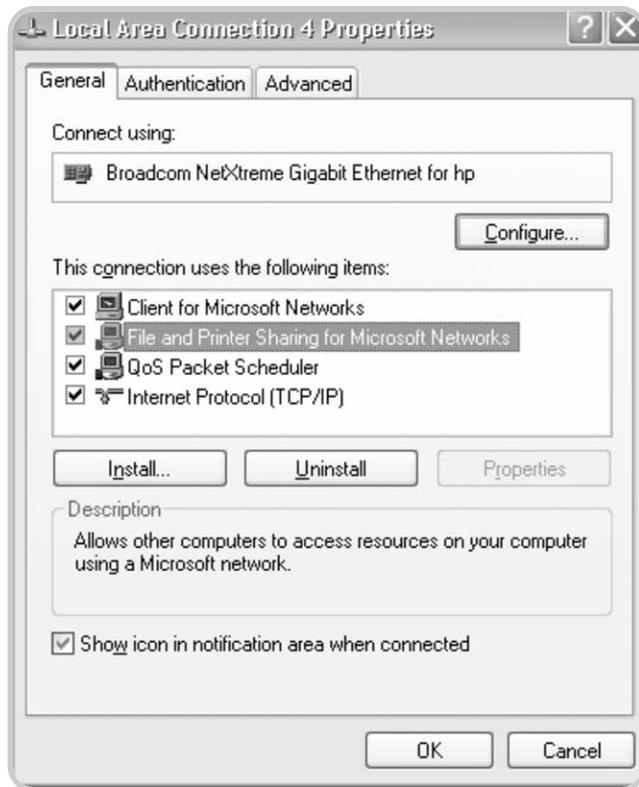
Figure 5. Use the Local Area Connection properties window in Windows XP to activate Internet Connection Sharing.
