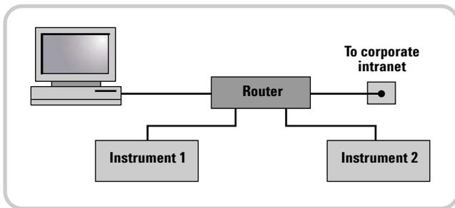
**Figure 2.** A test system that uses a router-based private, protected LAN.
