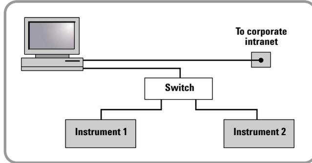
Figure 4. The PC-based solution, with two LAN cards in the PC and a switch to connect the instruments.
