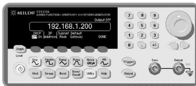
**Figure 6.** The IP Setup menu of the Agilent 33220A function/arbitrary waveform generator makes it easy to set the IP address, subnet mask and default gateway.
