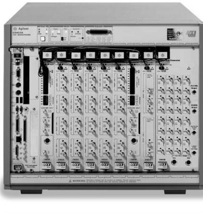
Figure 1. A typical VXI system
