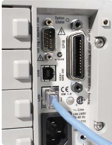
Figure 3. Many of today’s instruments have multiple I/O ports: the Agilent 34980A switch/measure unit shown here is equipped with GPIB, LAN and USB ports.
