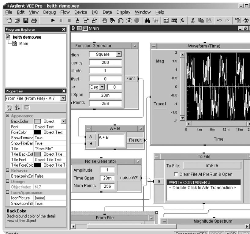
4. **Rapid prototyping**—With the intuitive nature of a graphical programming language, it can be easier to quickly build a prototype of your system. The prototyping capability is less useful when dealing with a large test system, but prototyping can aid development of systems of any size.<sup>12</sup>
