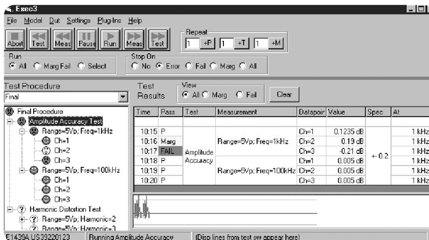
One of the most important features of a test executive is its test sequencer. As shown on the left side of Figure 11, the test sequencer is a sequence of tests that can be manipulated in design mode. Various test executives provide different levels of flexibility in this sequence, such as “test looping.”
