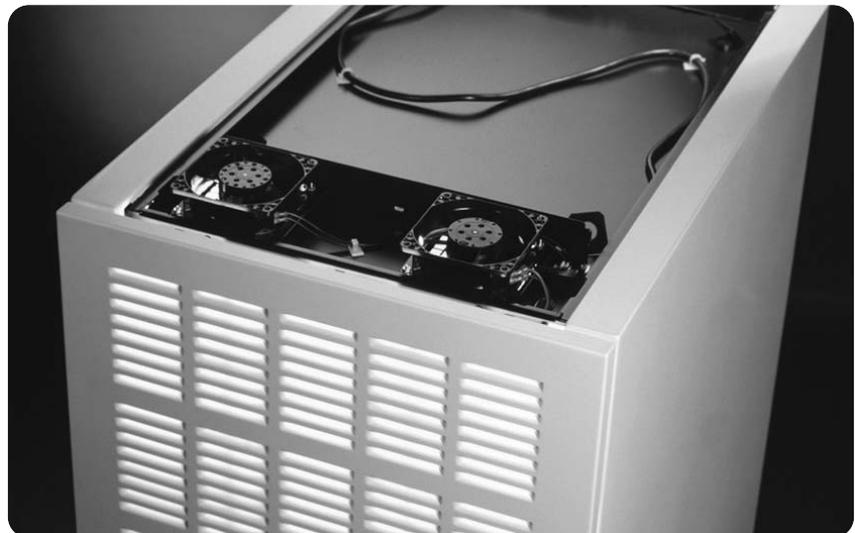
clearance around instruments. In general, place your deepest instruments at the bottom of your rack. If you place a full-depth, full-width instrument in the middle of the rack, you block airflow to the instruments below it.
