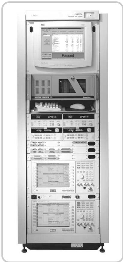
Figure 1. PC and test instruments in a rack.
