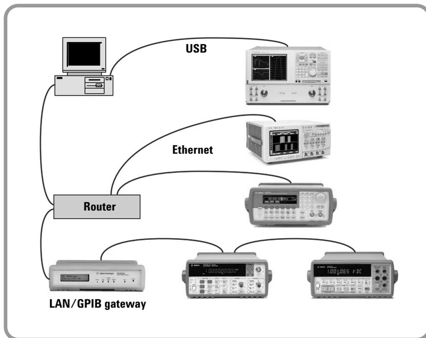
**Figure 4** An example test system that utilizes a PC, several instruments, a LAN router, a LAN/GPIB gateway and three types of I/O.
