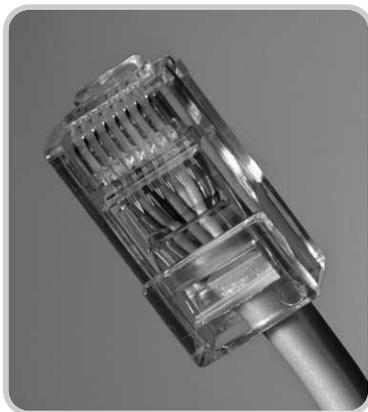
Figure 2. A CAT5 LAN cable with RJ-45 connector.
